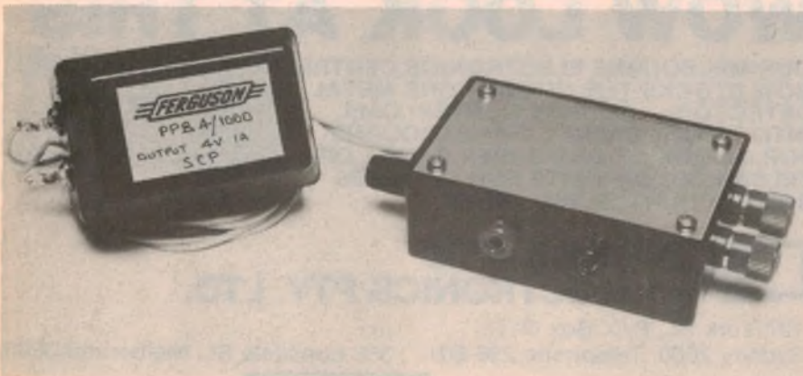
Power for the In-Circuit Component Tester is derived from a 4V AC plugpack supply. The device can test resistors, capacitors, inductors, diodes and transistors.
