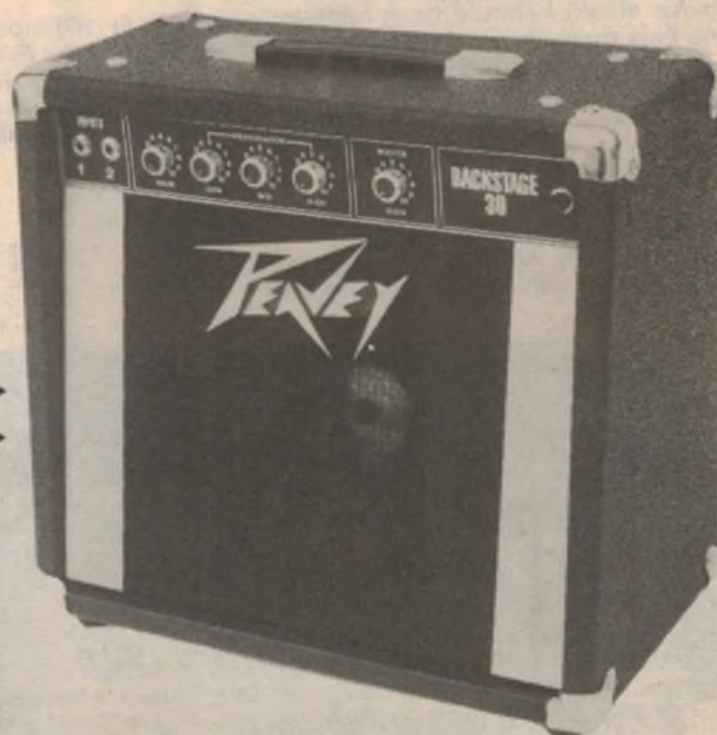
RIGHT: The Peavey Backstage 30 is typical of amplifiers in the lower price range, designed for home or rehearsal use rather than hard-driving rock concerts. It is a combination unit with an output of 18W, and incorporates a 30cm speaker and a single channel equaliser. (Australis Instruments Pty Ltd).
