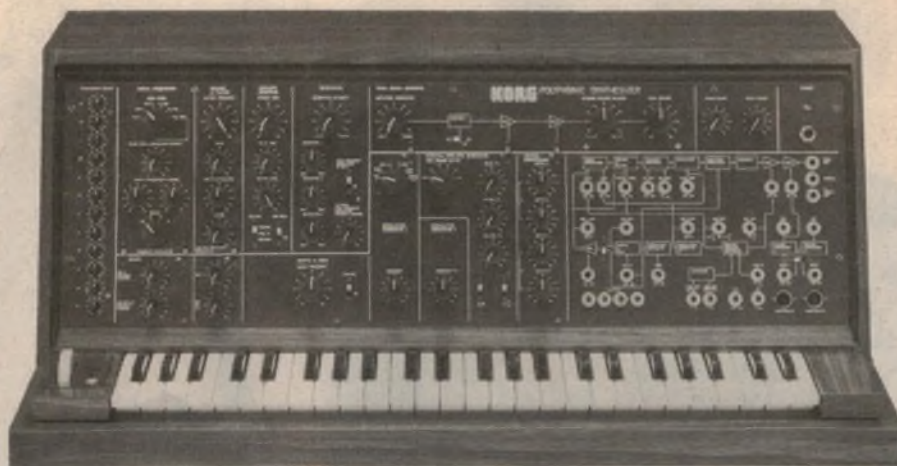
The Korg PS-3100 polyphonic synthesiser is one solution to the problem of playing notes simultaneously. It has a separate VCO, VCF, VCA and Envelope Generator for each of the keys of the keyboard. (Farrells Total Music Pty Ltd).
