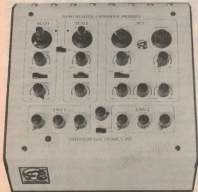
LEFT: The Oberheim Synthesizer Expander Module is a complete synthesiser voice module and the basic building block of Oberheim's polyphonic synthesisers (Orbital Music Pty Ltd).
