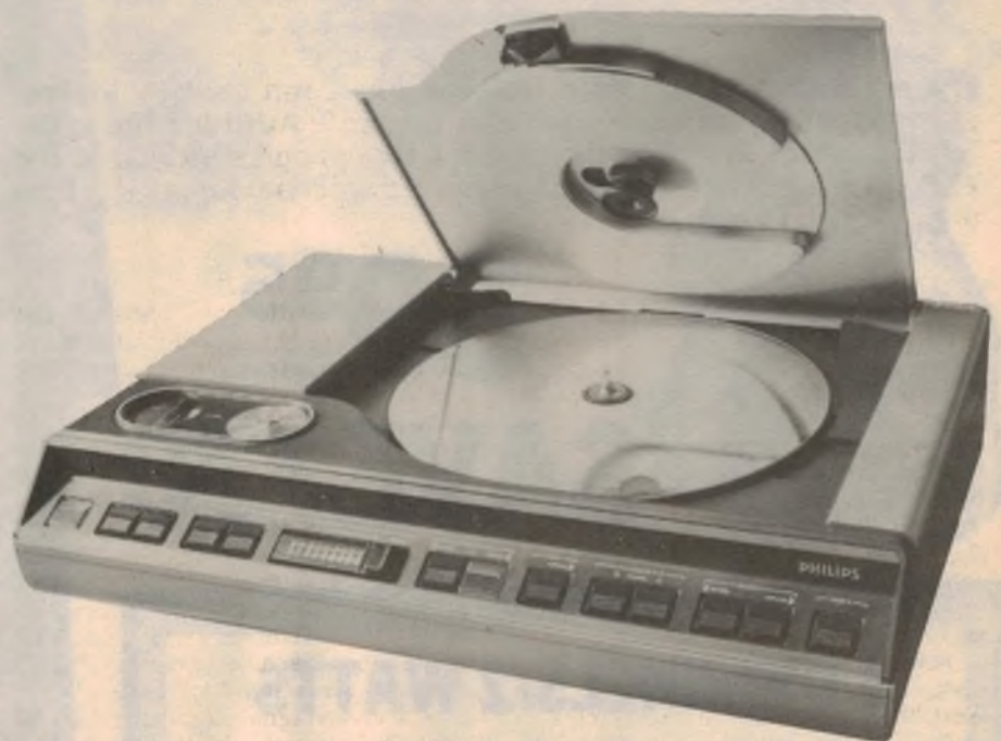
Pushbutton control and ease of operation are the main features of the VLP player. The unit is about the same size as a video cassette recorder.
