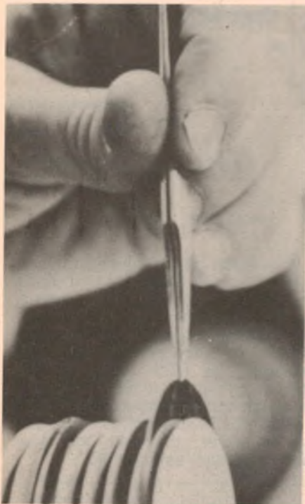
Left: To change the electrical properties of the silicon, wafers are inserted in a quartz rack and inter-leaved with the appropriate dopant. The wafers are then heated in a special high temperature diffusion furnace (above), causing the atoms from the dopant to migrate to the silicon.
