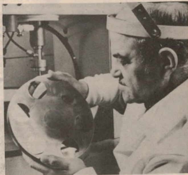
NBS technician Louie Robinson holds a polishing disc with six silicon wafers mounted on it.
