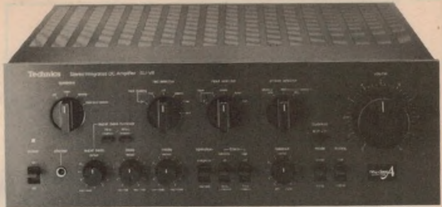
For those who want power to spare, this "New class A" SU-V8 retails for around $700 and delivers 105W+105W into 8 ohms or 140W+140W into 4 ohms, both channels driven; this, continuous, for all frequencies between 20Hz and 20kHz. THD at full power into 8 ohms, 20Hz to 20kHz, is 0.007%. Maximum available power is 160W+160W.
