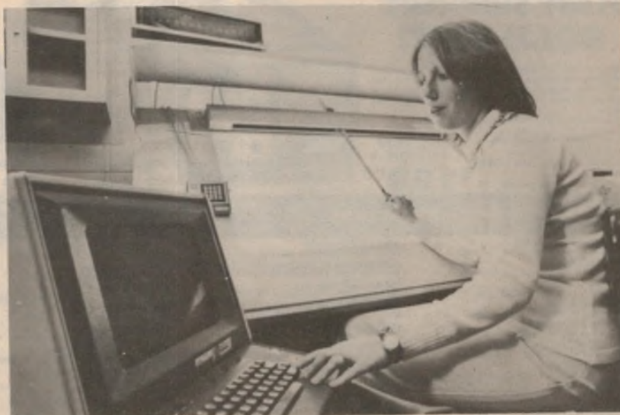
Kerry Fischer of the NBS semiconductor processing facility uses a digitiser which converts a test design into a set of co-ordinates stored in computer memory.
