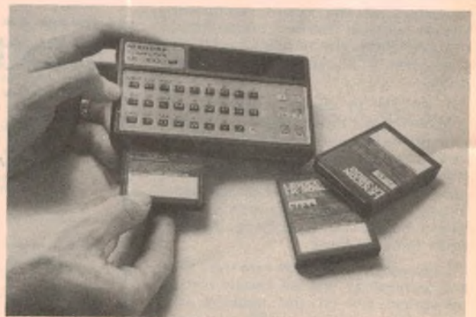
Nixdorf unit ($US140) accepts language modules ($US60) or interface connectors ($US150) for attaching it to a computer.
