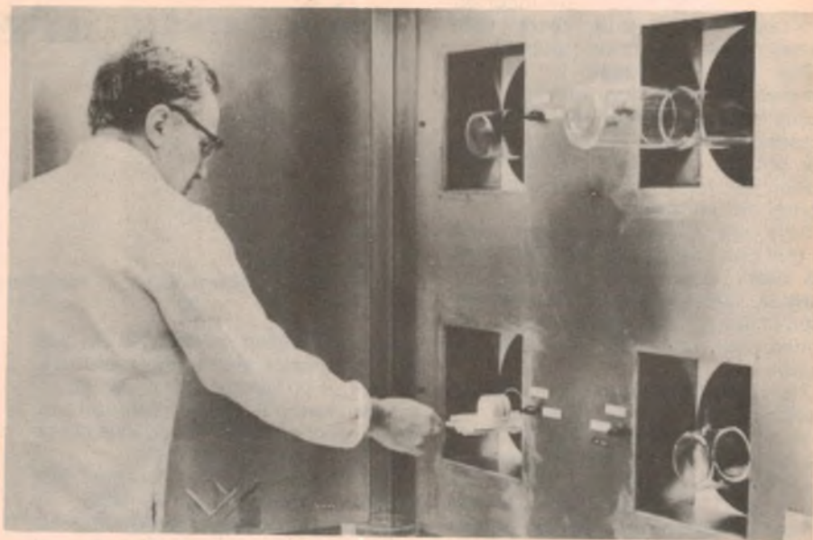
Left: To change the electrical properties of the silicon, wafers are inserted in a quartz rack and inter-leaved with the appropriate dopant. The wafers are then heated in a special high temperature diffusion furnace (above), causing the atoms from the dopant to migrate to the silicon.
