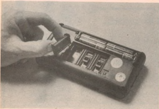
The Craig translator accepts up to three modules at once for cross-translations and phonetic spellings. US price is $200.
