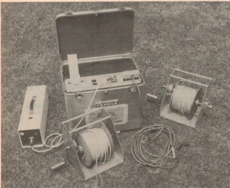
Sirotem consists of two units; a transmitter/ receiver and a battery pack.
