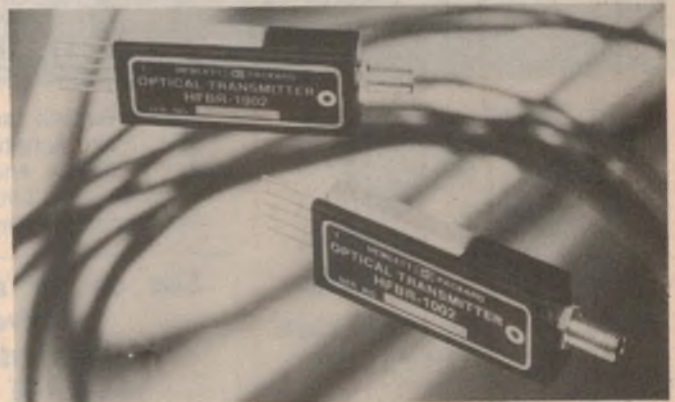
New HFBR-1002 fibre-optic digital transmitter from HP makes 1km data links possible.
