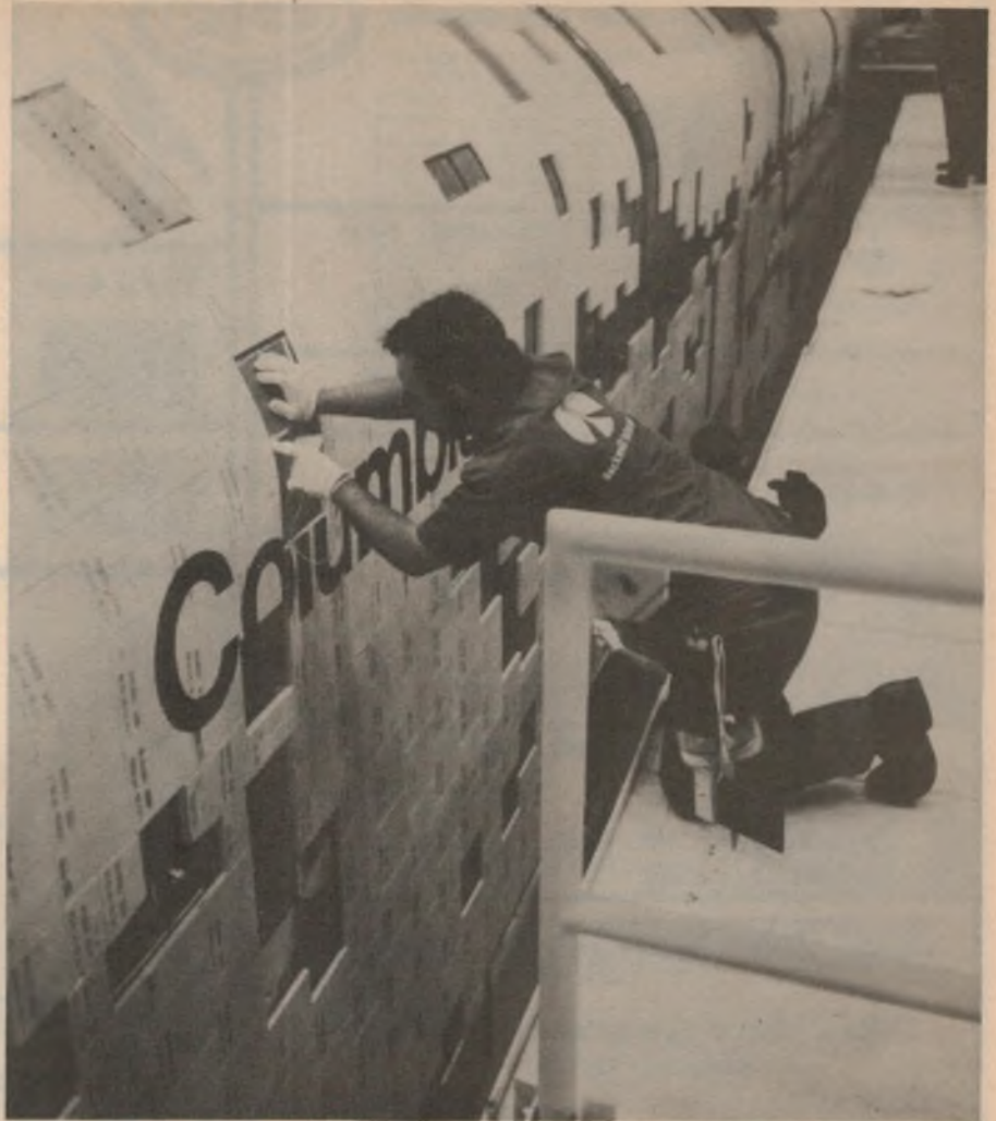
A worker carefully applies white tiles to the fuselage of the Shuttle Orbiter "Columbia". The Orbiter underwent a successful mock flight last December in which ground-based computers tested the responses of the on-board computers.
