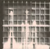
NARROW DISPERSION: Analyzer sweeps \pm 0.5 MHz from selected frequency (1 MHz span)
