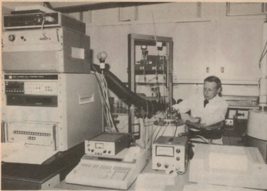
Dr Bryan Taylor amidst the tools of his trade — the most precise calorimeters available. The calorimeters can sense miniscule quantities of heat which flow from the reaction of metal alloys with hydrogen. Information derived from the measurements will enable the research team to improve hydrides by developing better alloys.
