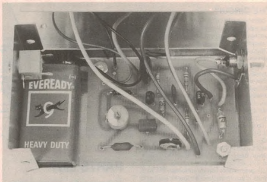
Above: view inside the prototype. Note that this unit is powered from its own 9V battery and has not been wired to accept an external plugpack supply.
