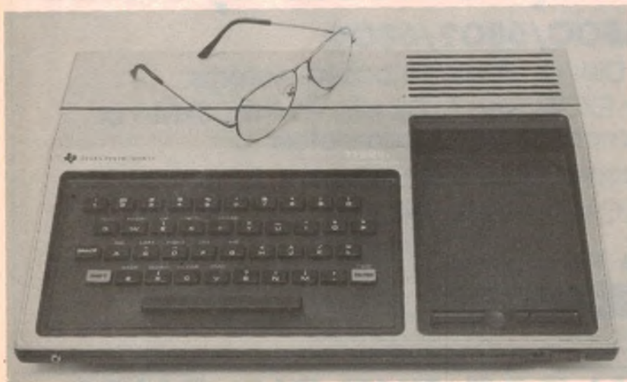
Size of the keyboard console is evident in comparison to the spectacles on top. On the right side is the slot for software modules, and the volume control.
