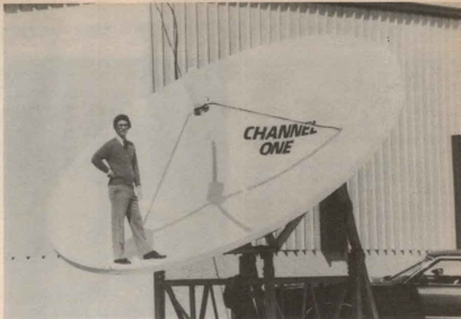
Fred Hopengarten, President of Channel One Inc. poses in a 16.4ft diameter dish designed to receive television signals direct from a satellite in stationary orbit at a height of 22,300 miles.
