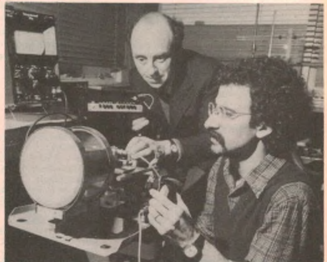
A polythene lens focusses a microwave beam in this prototype collision avoidance radar system for cars.
