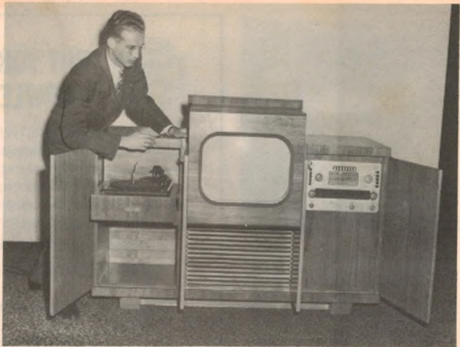
The style of the 40s – a 1947 "Hampshire model Du Mont 20-inch television receiver" from the USA. Included in the same console were an AM/FM radio and an automatic record changer.
