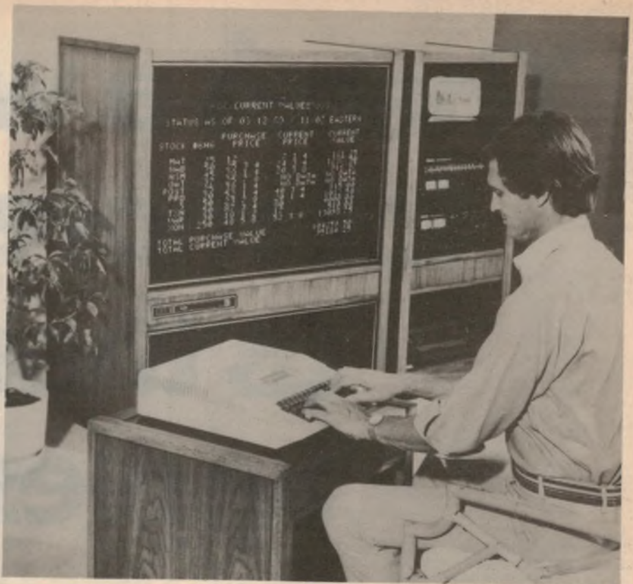
JUST RELEASED by General Electric, the Widescreen 3000 Home Television Centre features a big rear-projection 115cm diagonal flat screen and comes with full remote control facilities. Pictures are projected via a 3-lens system from three 12cm CRTs at the rear. GE says that the new receiver makes an ideal display device for home computer systems. Price in the US is around $3,500!
