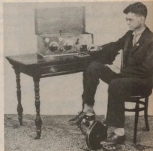
Traeger as a young man with an early model pedal generator & Morse code transceiver. (Photo courtesy Museum of Applied Services, Sydney).
