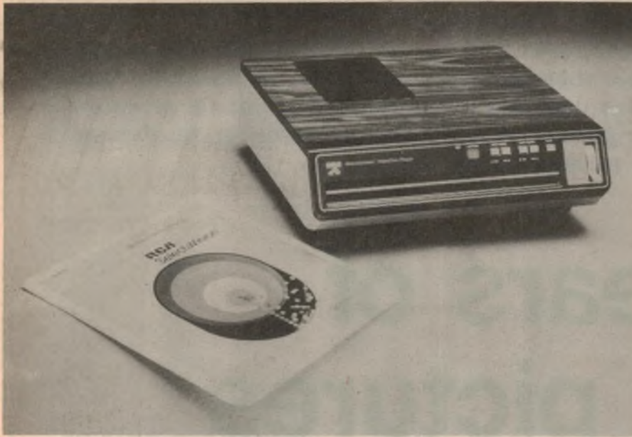
Left: RCA's Selecta Vision player. As with the VHD system, the record is inserted with its caddy through a slot in the front of the player. The player then extracts the record and returns the caddy before beginning to play.
