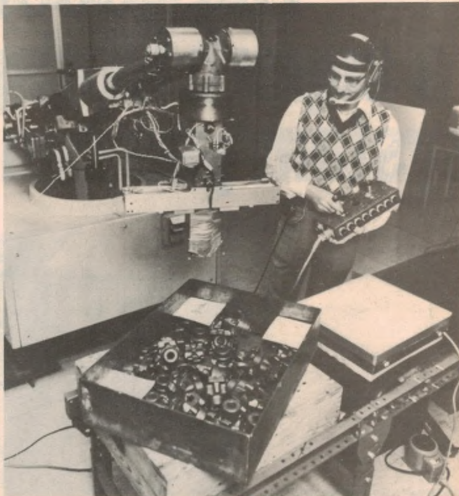
Overall view of the "intelligent" robot developed at Stanford Research Institute. Here an operator trains the system to identify the corner positions of a bin.
