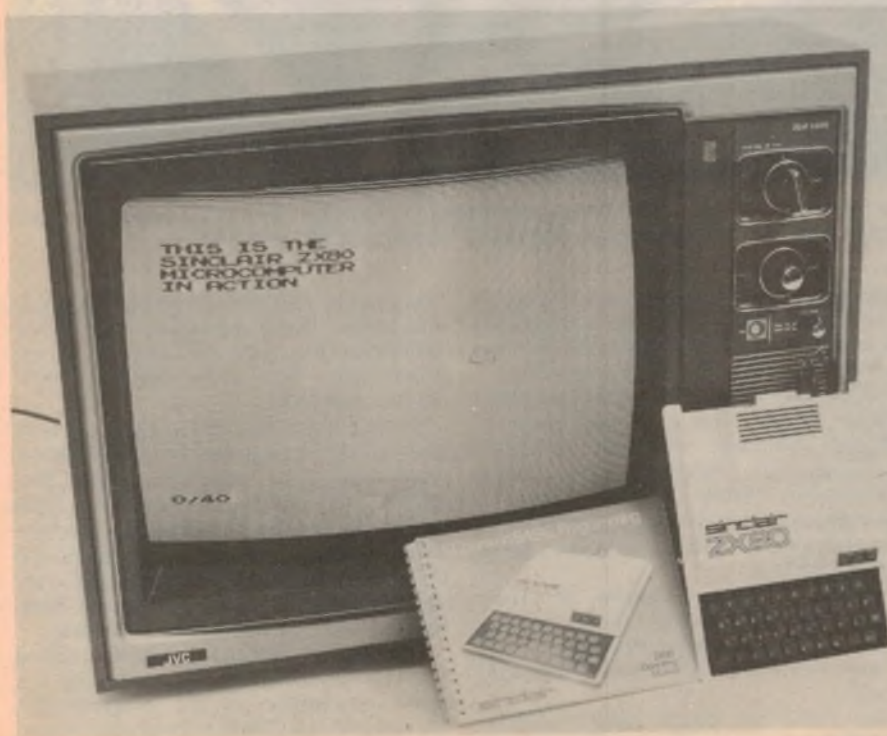
Left: the Sinclair ZX80 in action. The ZX80 is easily held in one hand, yet features full BASIC operation and single keystroke functions.
