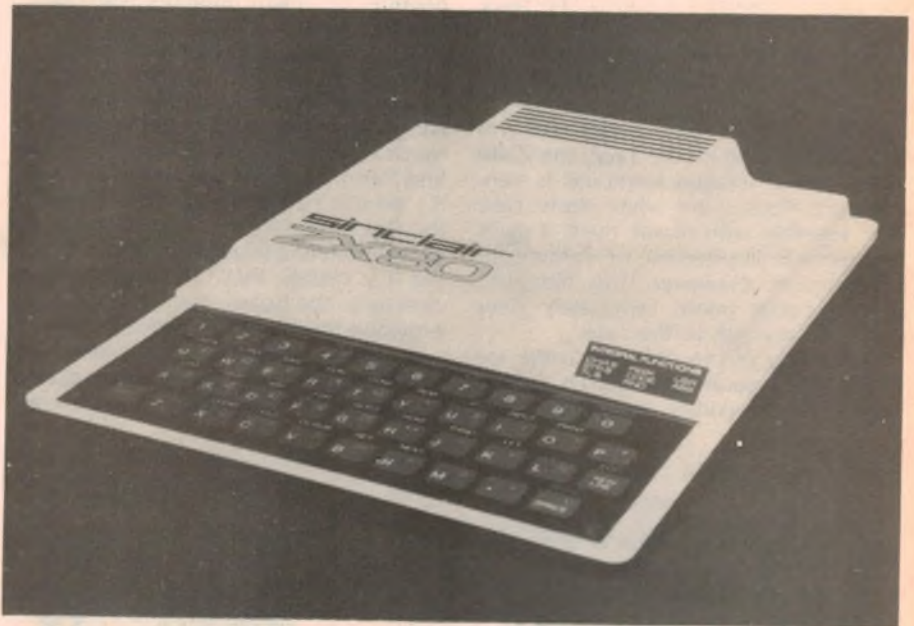
A close up of the ZX80 personal computer. Features include a touch sensitive keyboard, 1K of RAM, and an internal RF modulator for VHF Channel 1.
