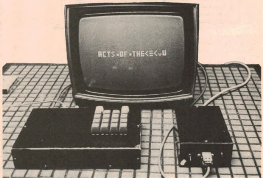
The author's DREAM 6800 displaying a radioteletype message. The computer itself has been built in an aluminium box to prevent RF interference. Its power supply is the smaller unit on the right. The symbols following "the" on the display are carriage return and line feed indicators.
