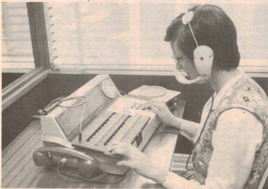
Above: a talking switchboard adapter for blind switchboard operators. It uses a microprocessor-based control unit to scan the status of panel lights on the switchboard, and generates audible commands using synthesised speech.
