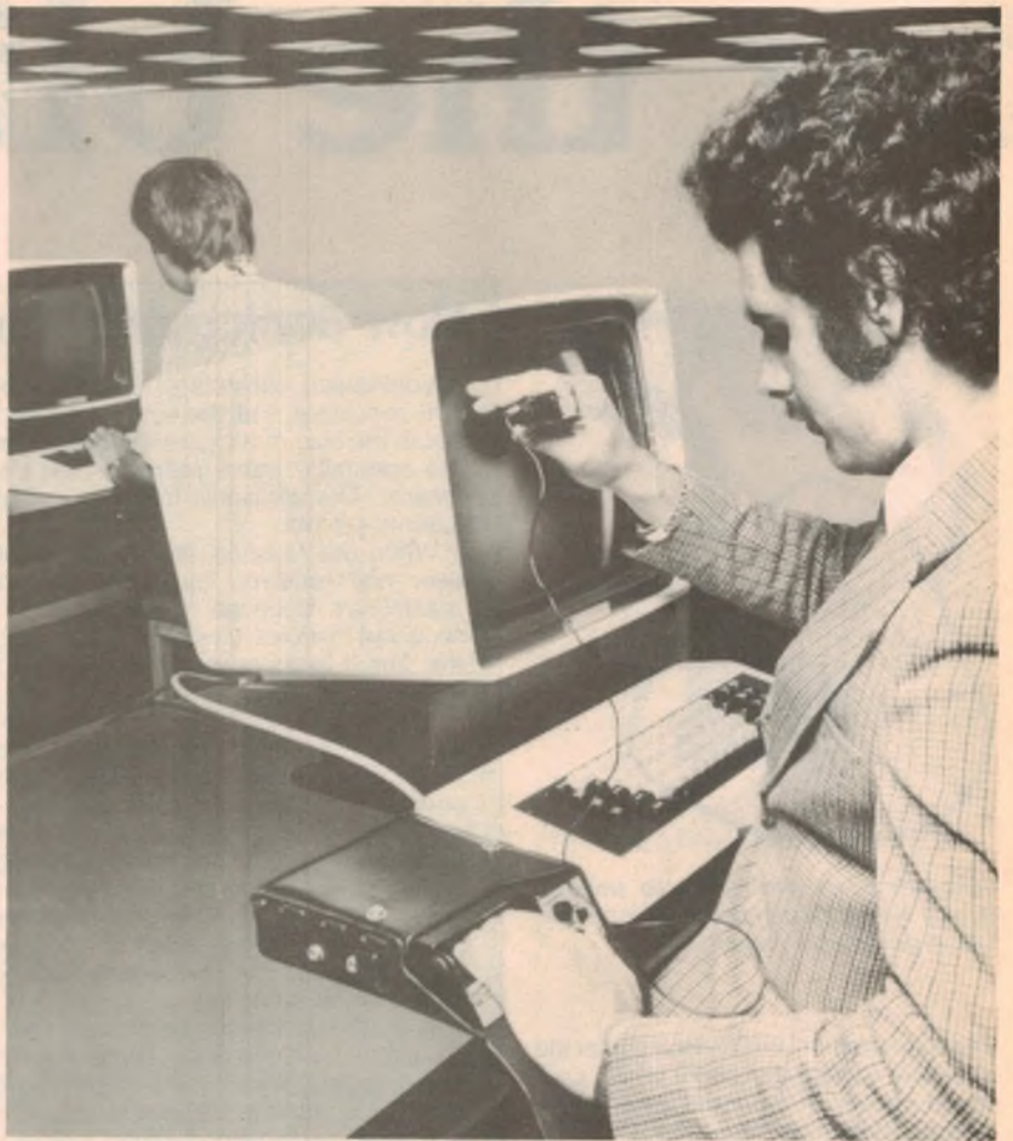
A blind computer operator uses an Optical-to-Tactile Converter – the Optacon – to read a CRT terminal. The machine converts the image of a letter into a pattern of vibrating rods which are read with the index finger of the left hand.
