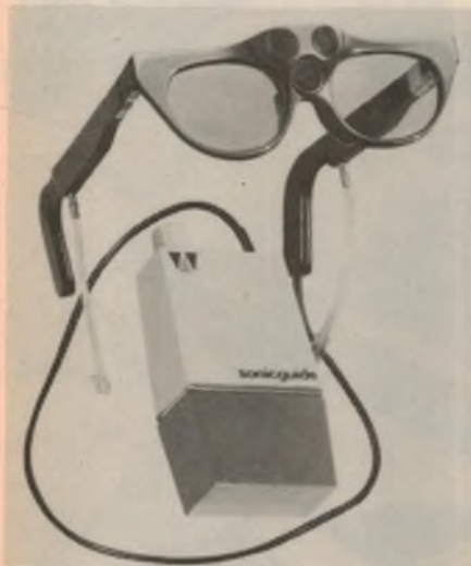
Sonicguide uses ultrasonics to provide the user with distance and position information on nearby objects.
