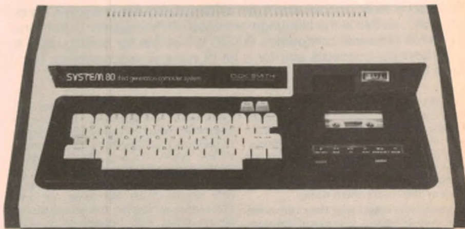
On the improved System-80 the right hand SHIFT Key has been replaced by the BACK SPACE and new TAB keys.
