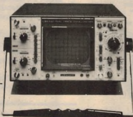
Model LBO-520. A dual trace oscilloscope with a 30MHz bandwidth a 5mV/cm sensitivity. Delay triggering and a 130mm, post acceleration, CRT produces a bright, sharp display. Display offers chop, act, add and subtract, Ch1, Ch2, also X-Y:
