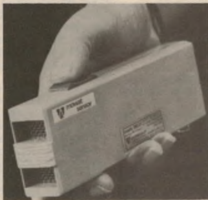
The Visualek reading aid. It displays magnified images on a TV screen so that partially sighted people can read and write.
