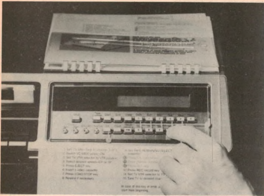
Flip cards fit over buttons to aid programming the microcomputer in Sharp's VC-6800. LEDs on the deck's tape-remaining selector (left) light up so you can tell if there's enough to finish recording a program.
