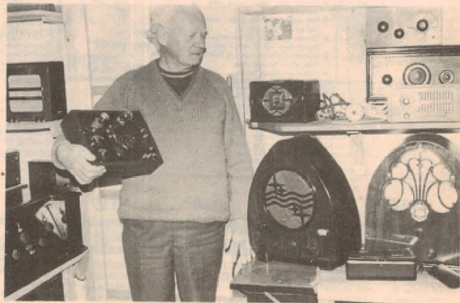
ABOVE: Keith McIlraith holds a radio receiver he made about 1925. It used two 01A valves and a crystal detector, and gave good reception on headphones. Other receivers in this photo and the photo at left include: 1923-24 Crossley (USA) 5-valve; 1931 Philco (USA); 1929 Philips 4-valve; Astor (Aust.) 5-valve; 1935 Cromwell (NZ) 5-valve; 1934 Stewart Warner (USA) 5-valve; 1932 Decca (UK) 4-valve; 1936 Stromberg Carlson (Aust.) 5-valve; and a 1938 Columbus (NZ) 7-valve.
