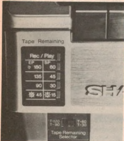
Flip cards fit over buttons to aid programming the microcomputer in Sharp's VC-6800. LEDs on the deck's tape-remaining selector (left) light up so you can tell if there's enough to finish recording a program.
