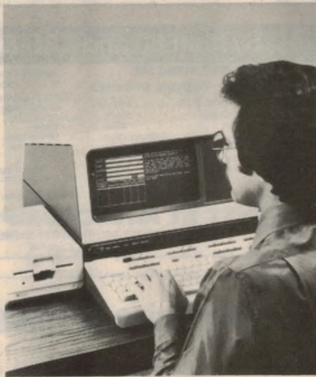
Hewlett-Packard's 2642A CRT Terminal is offered with flexible mini-disc option for local mass storage.
