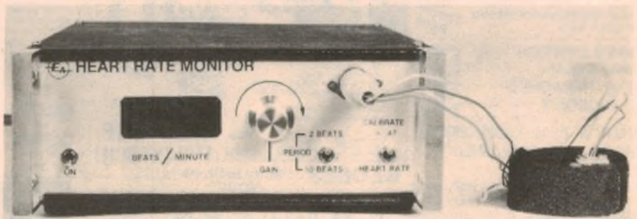
Pictured above is the Heart Rate Monitor together with the wrist-strap sensor. It can be used during any stationary exercise such as pedalling an exercise bike, as pictured at top left (Photo courtesy of "Vital" magazine).
