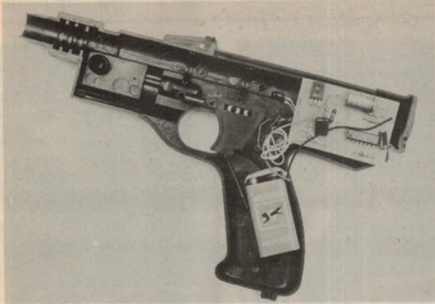
The completed target game transmitter inside a plastic gun. Although the PCB layout differs from the overlay, the two are electrically identical.
