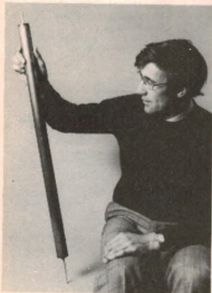
A sodium-sulphur cell. It measures 850 x 38mm and has an EMF of 2.08V.
