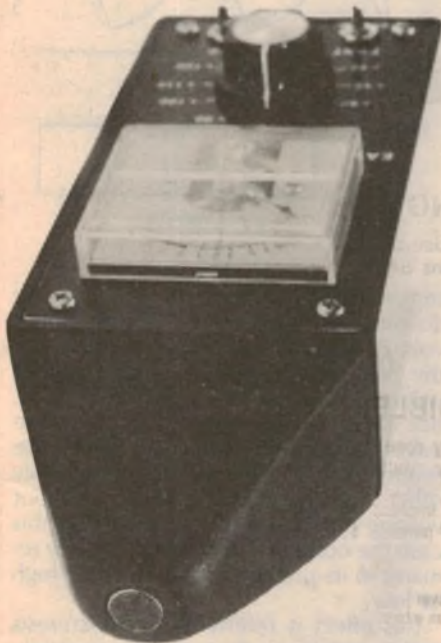
At left is a view of the Sound Level Meter showing how the microphone insert is recessed into the nose cone, which is shown in perspective view in the diagram above. Also shown on this page is the full-size artwork for the PC board and front panel.
