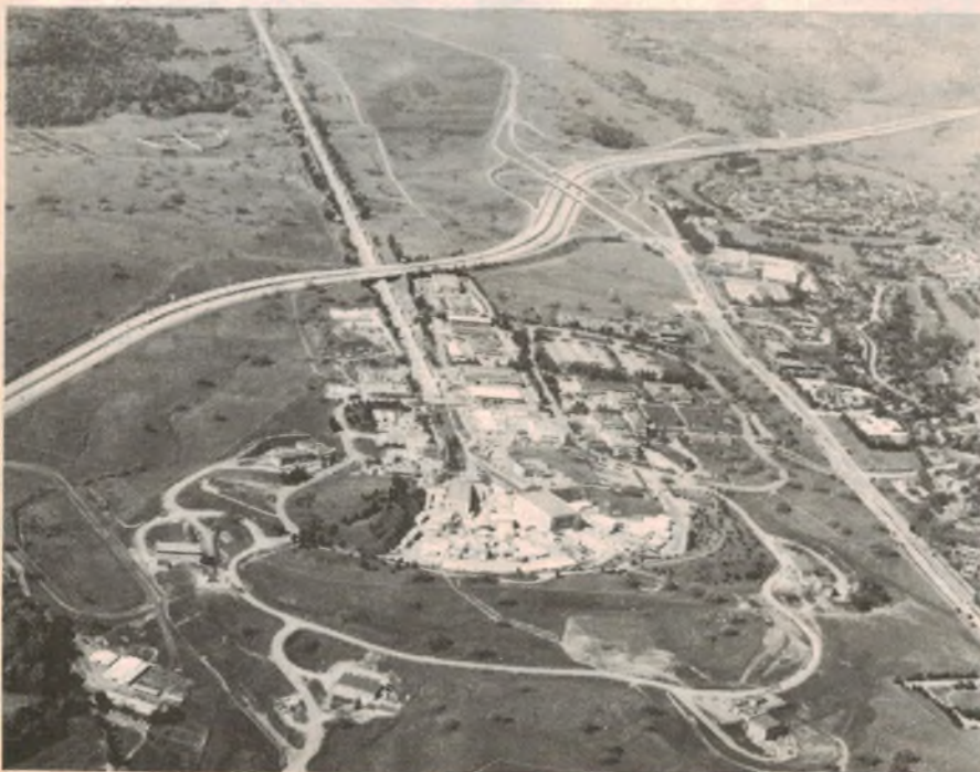
LEFT: the 3.2km linear accelerator disappears into the distance from its cluster of experimental halls. The PEP ring is in the foreground, adjacent to the access road.
