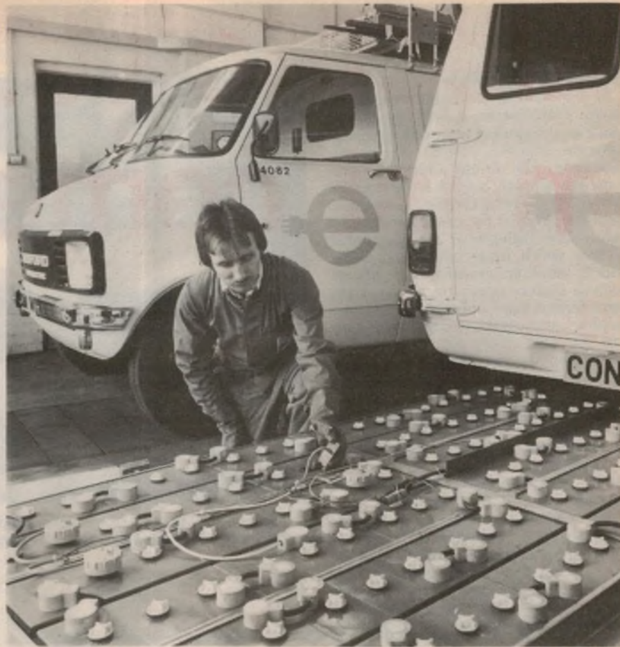
Lucas/Bedford electric van with detachable battery pack withdrawn for maintenance. (Photo courtesy Lucas Industries Ltd.)
