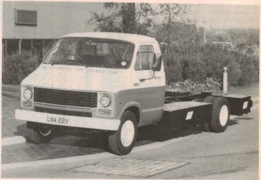
The Dodge 50 Electric Vehicle developed by Chloride Technical Ltd. Battery packs can be seen to the side and to the rear of the vehicle.
