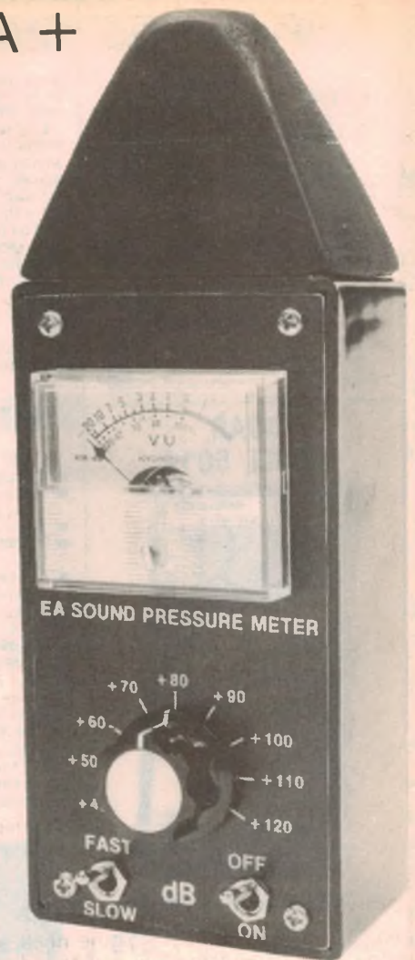
Our Sound Level Meter measures sound pressure in nine ranges with fast or slow response.
