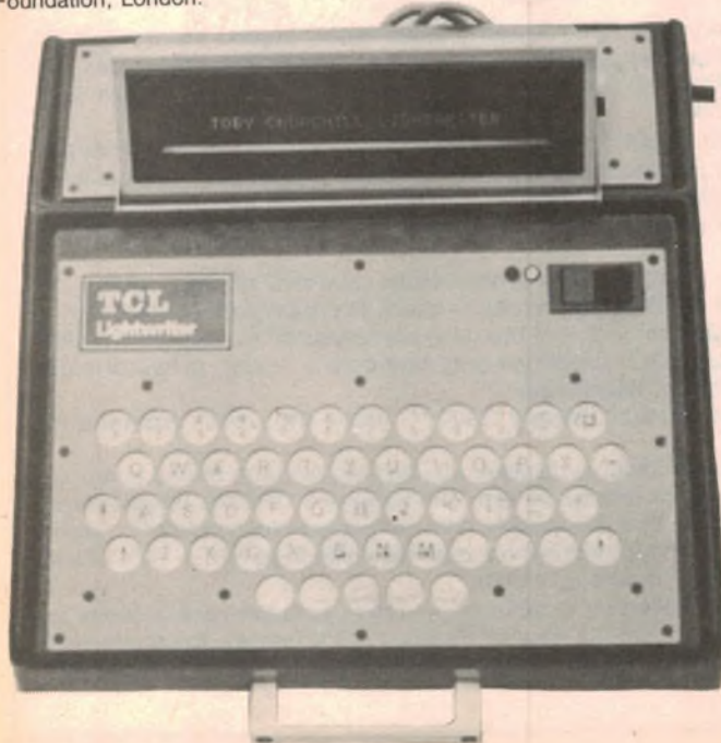
LEFT: phrases can be displayed on the Lightwriter screen by operating the typewriter-like keyboard. Screen is detachable.
