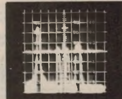
NARROW DISPERSION: Analyzer sweeps \pm 0.5 MHz from selected frequency (1 MHz span)
