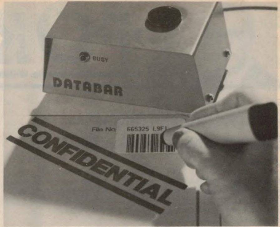
Movement of sensitive documents and files can be monitored by bar code readers.
