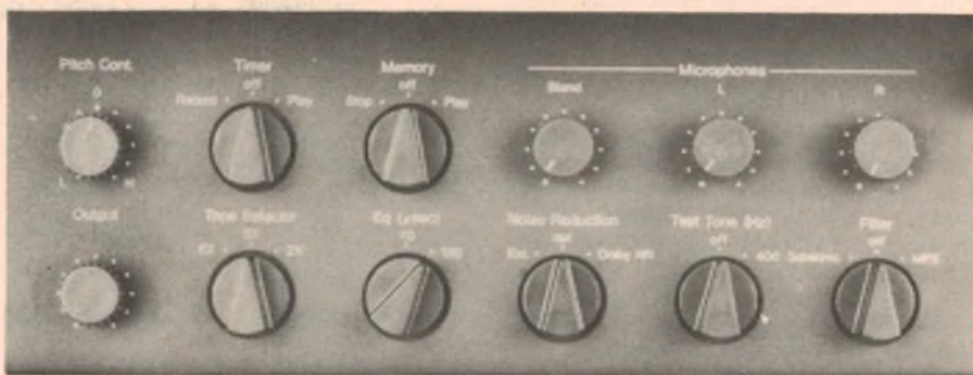
This is the control panel hidden by the flip-up door on the front panel of the 700ZXL.
