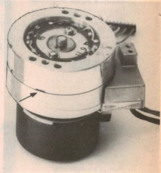
The video motor/drum/head unit from a modern National Panasonic VHS home video deck. The tip of one head is indicated by the arrow.
