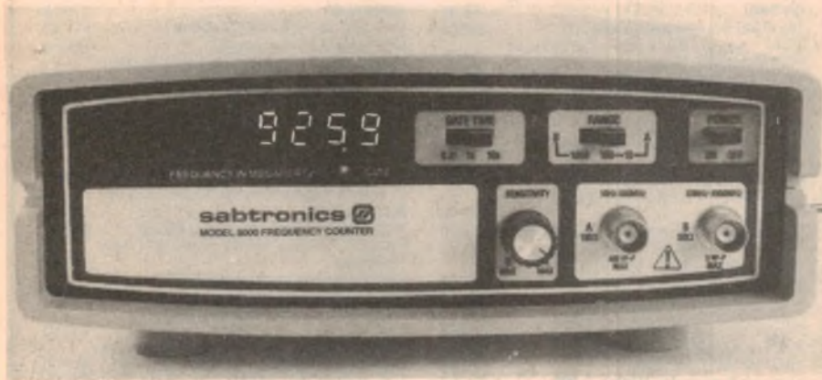
The Sabtronics 8000 has a 9-digit readout but is shown here with a 4-digit reading.
