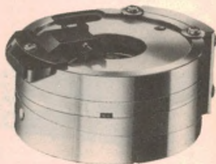
Fig. 1: The video head drum unit from a Sony Beatmax VCR. The centre section carrying the two video heads rotates at 1500rpm. The tip of one head is just visible in the tiny rectangular aperture in its lower edge. As the tape moves slowly around the spinning drum from upper left to lower right, the heads lay magnetic tracks obliquely across it.
