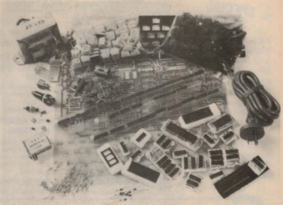
This is what the standard kit will look like when you unpack it. Not shown is the tape cassette with interpreter plus an instruction manual.
