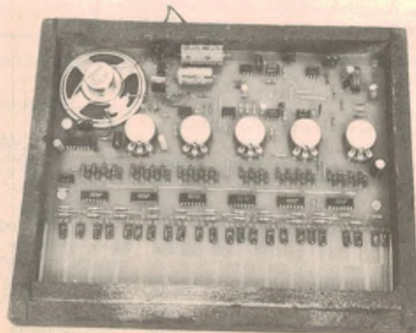
The completed prototype, fitted with a Scotchcal front panel. Photo at right shows how the PCB is mounted in the case.
