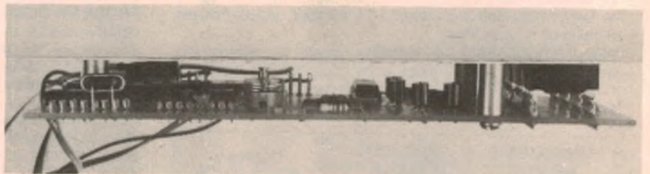
View showing how the PCB is attached to the front panel using brass spacers.
