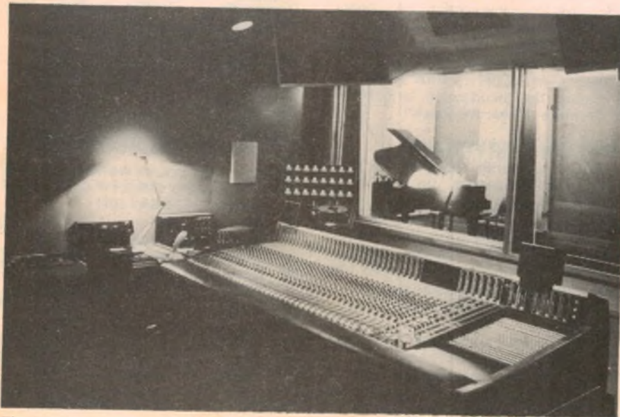
The Harrison 4032 console, serving the main music studio, can cope with 40 inputs and 32 outputs but provision is available to interlock both studios for complex tasks.
