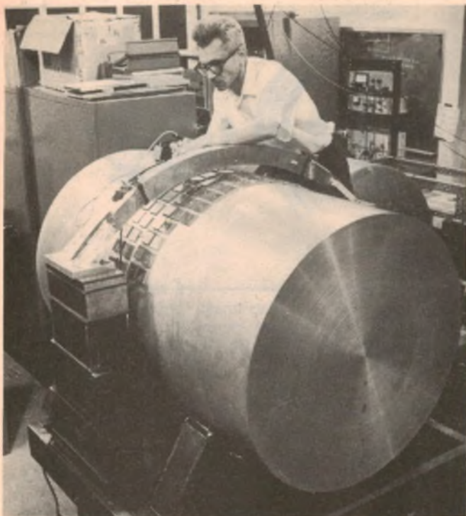
Dr Joseph Weber of the University of Maryland at work on his invention, the first gravity wave detector.
