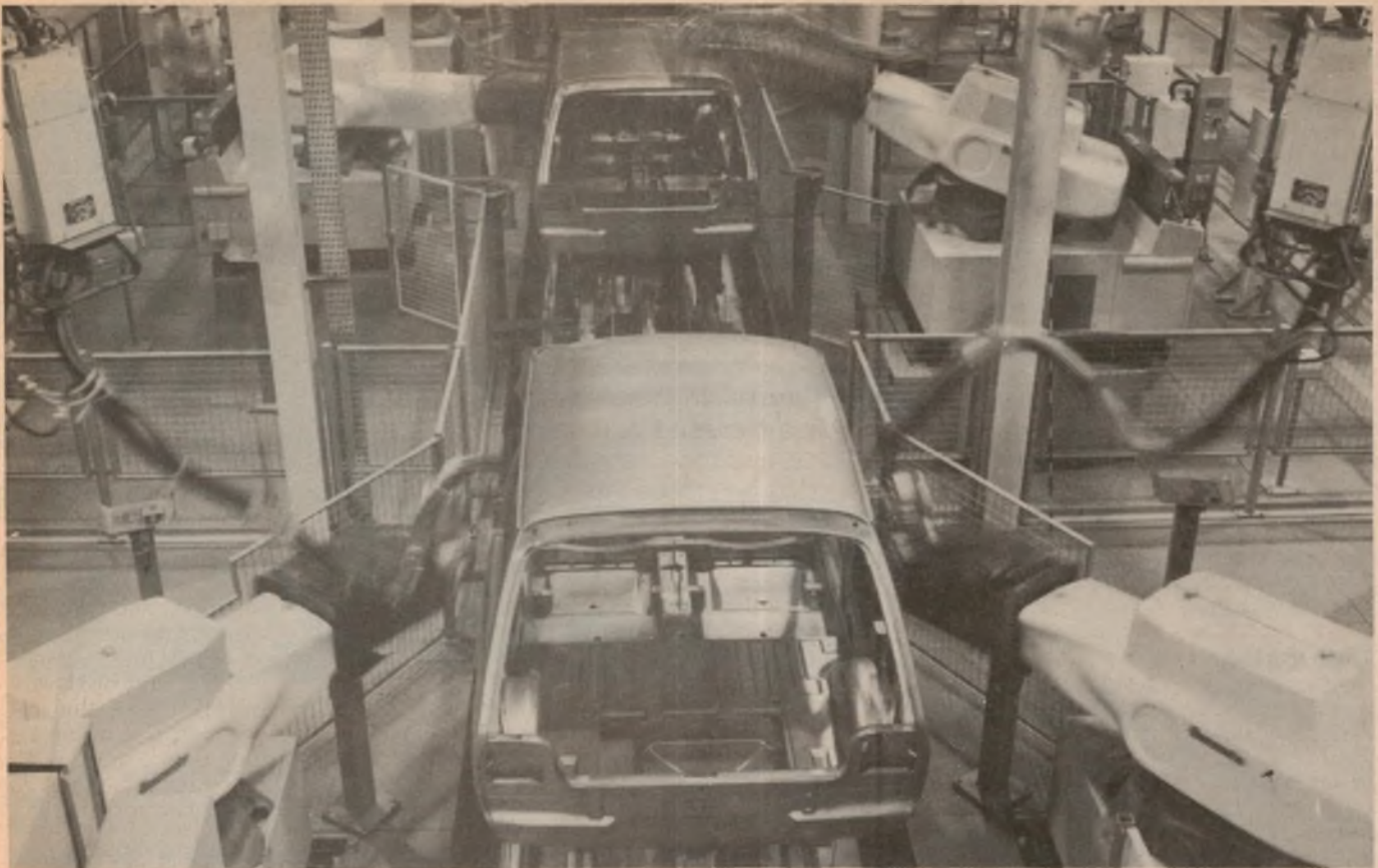
"Many robots make light work" – a robot welding line produces the new British Leyland Metro.
