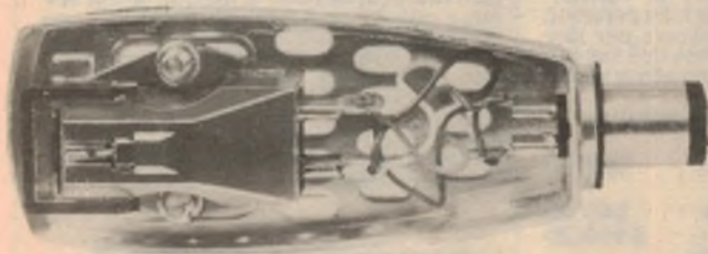
Shown above is the Ortofon MC20 MkII moving cartridge fitted into a headshell (normally not supplied). The MC20 has a flip-down stylus guard but the stylus assembly is not removeable.
