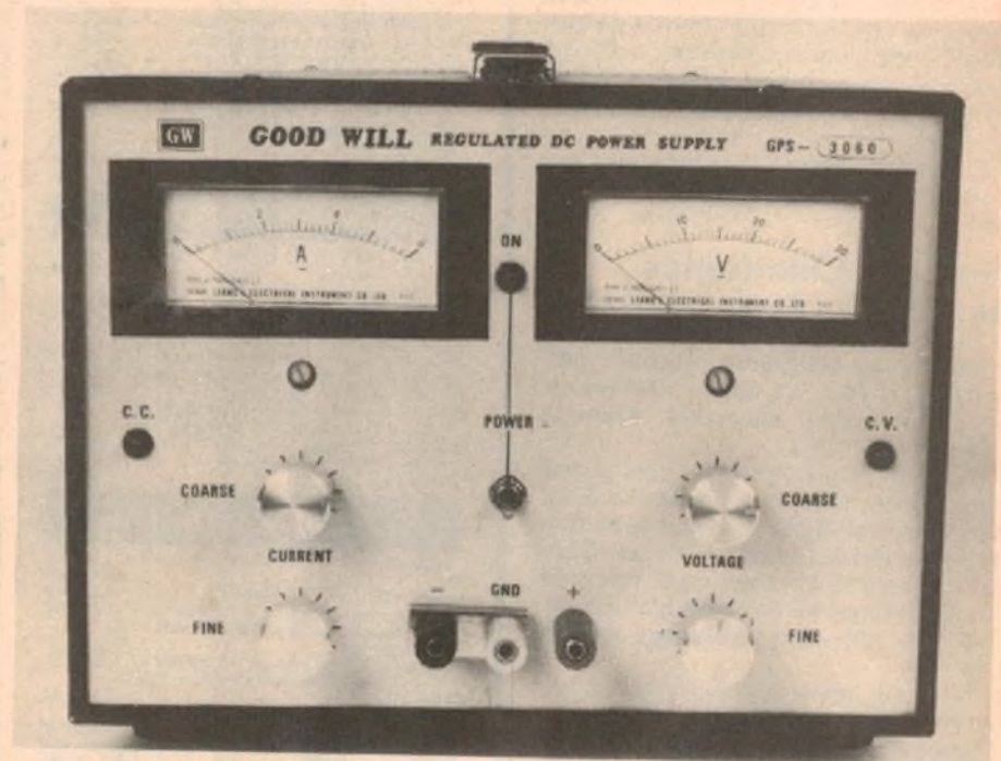
The Goodwill GPS-3060 — 0-30V output and adjustable current limit from 0-6A.
