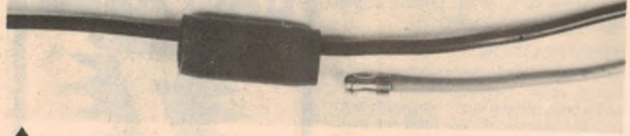
Above: the Audible Turn Monitor is connected into circuit using male "bullet" connectors and a 4-way female "bullet" adapter. Two adapters are required, one for each of the front lamps.
