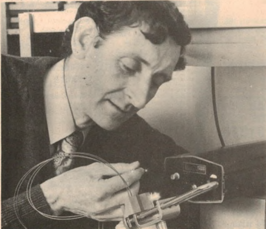
Computing Centre Manager Mr Brian Rowsell demonstrates that laser light shining into one end of the fibre optic cable is clearly visible at the other end.
