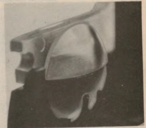
The split filter in the 640 camera which allows the photodiode to sense separately normal ambient light and infrared light reflected by the subject from flash.
