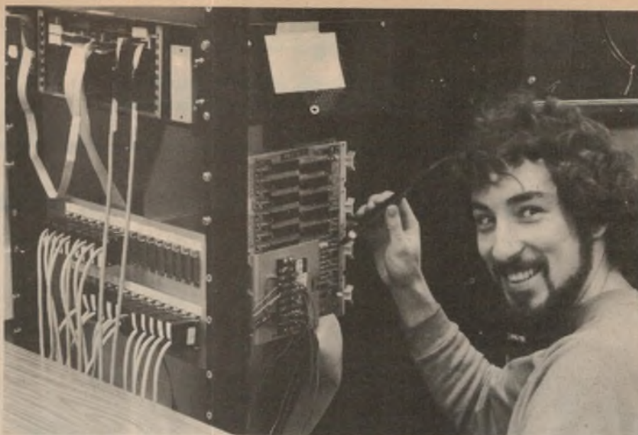
Technical Officer Mark Phillips checks a board which interfaces a node computer to terminals. All interfaces for the network were built at the University.
