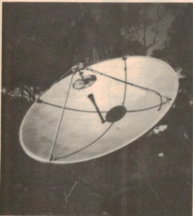
Three metre dish for the author's home-built satellite TV station came from a government auction. Other components were built at home, based on surplus equipment.
