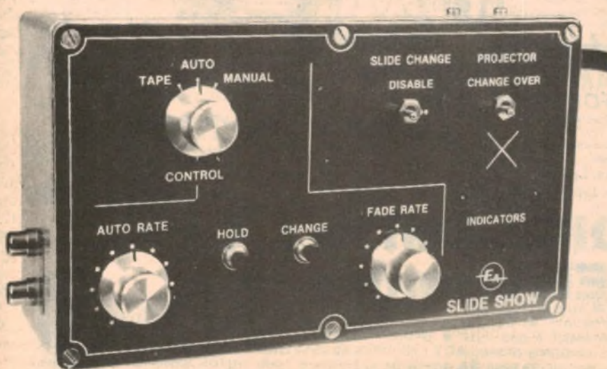
Slide Show can be used with virtually all types of automatic projectors. Features include three control modes, variable fade rate, and manual override.
