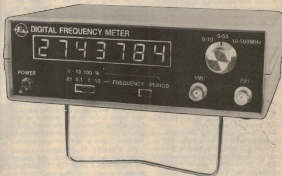
View of the prototype fitted with the optional tilting bail. The 1M \Omega input is used for the 0-10 and 0-50MHz ranges while the 75 \Omega input is used for the 500MHz range.
