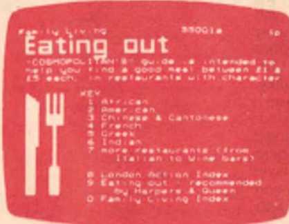
Viewdata systems store information in a central computer which can be accessed over the telephone lines.
