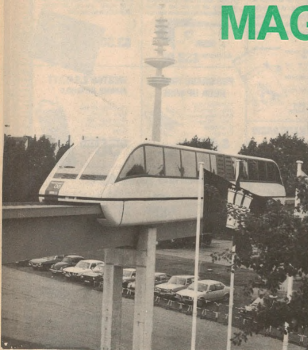
Above: the West German Transrapid 05. Results of tests on this vehicle will be used in the design of a high-speed passenger service over distances of 50 to 100 kilometres.
