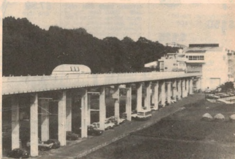
Above: the West German Transrapid 05. Results of tests on this vehicle will be used in the design of a high-speed passenger service over distances of 50 to 100 kilometres.
