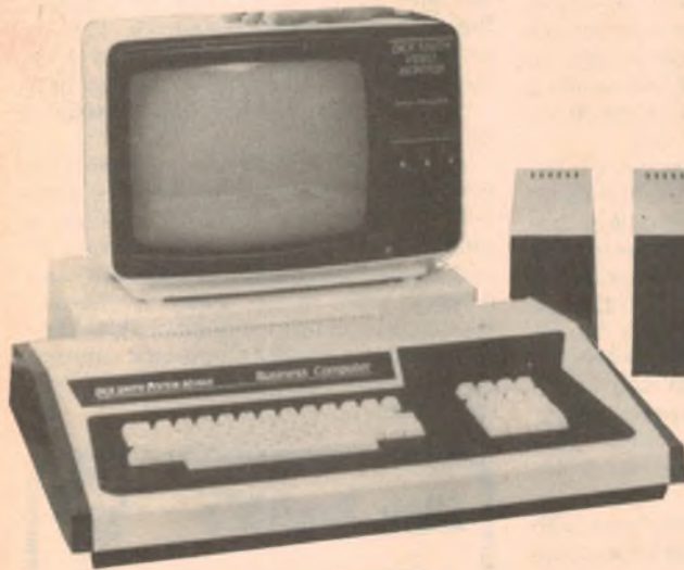
The Mk II System-80 is specially designed for business use. It is shown here with the expansion interface and a pair of Percom disk drives.
