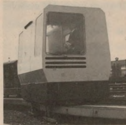
British Rail prototype maglev vehicle, 3.5m long and weighing 3 tonnes. Built in 1974, the vehicle proved the utility of magnetic levitation on steep gradients and tight curves at the Derby test track.
