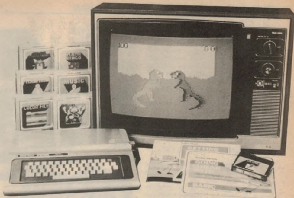
Shown above is the Color Computer console, games cartridges and manuals. The display is a standard PAL receiver, showing "Dinowars" in action.
