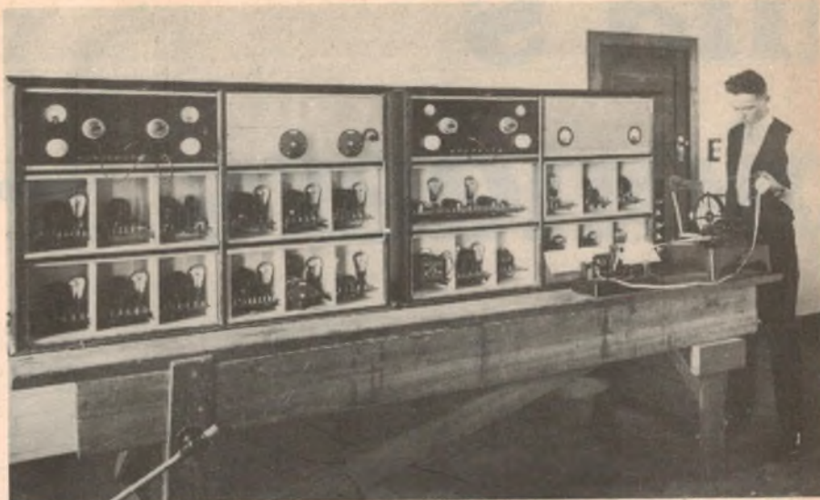
This "special 16 valve supersonic heterodyne receiver" was used at AWA's La Perouse station for reception of high speed morse code from Melbourne in the '20s.
