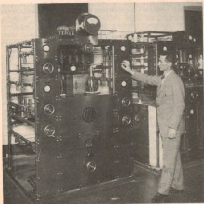
AWA engineer Sydney Newman with the company's experimental 20kW shortwave transmitter, Pennant Hills, 1928.
