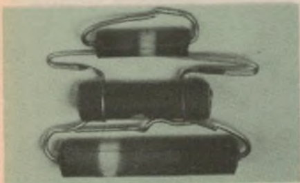
Impossible to envisage: modern equipment designed around the bulky resistors of yesteryear. The carbon types were none too rugged, either, and subject to drift.
