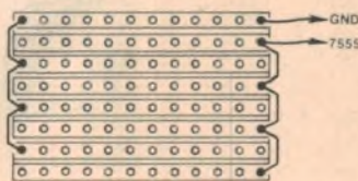
This diagram shows how the stripboard touch plate is wired.
