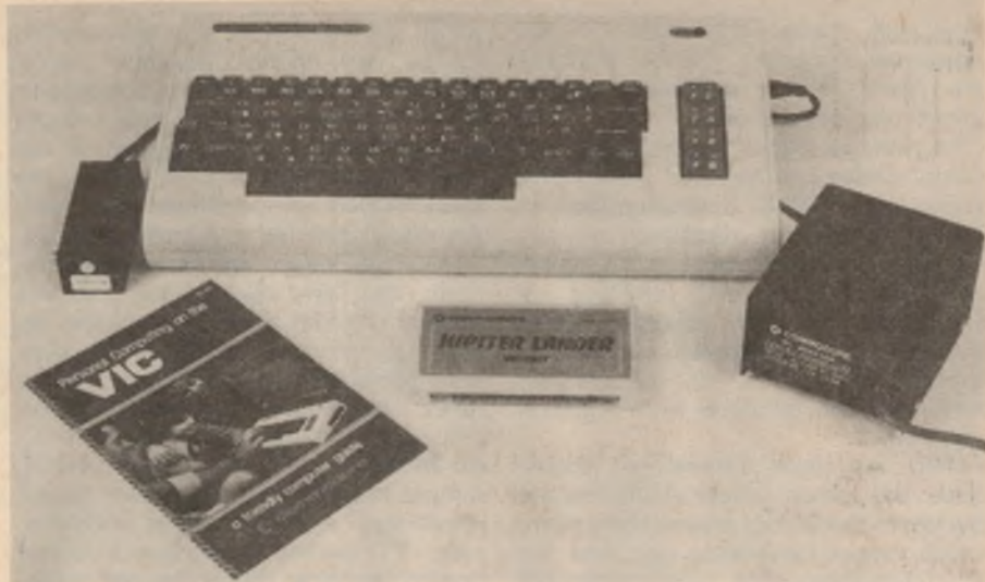
Another view of the system, showing the separate power supply (right) and video modulator (left of the console) and a program cartridge.
