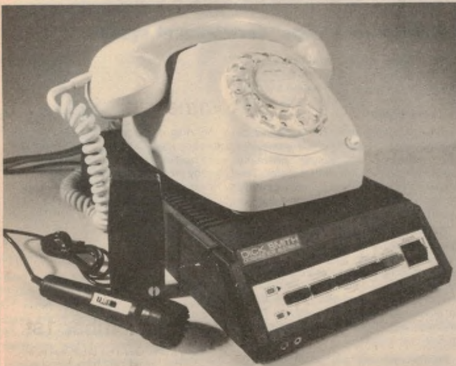
Telephone answering machine from Dick Smith Electronics uses two microcassettes, one for pre-recorded message to caller and one for recording incoming messages.
