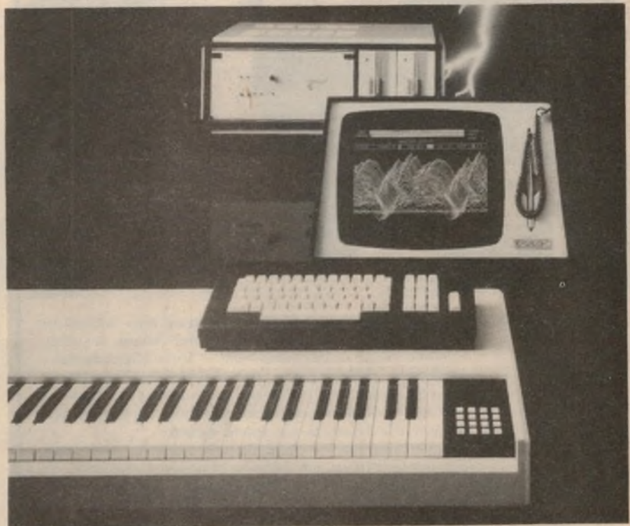
From the rear: the central computer unit including audio circuitry and floppy discs; the VDU with light pen; the computer style keyboard; the 6-octave music keyboard. The small numeric key pad at the front-right can be used as a tone selector — in the manner of organ stops — for stage performances.
