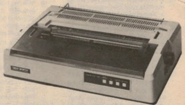
C-Itoh FP-10 daisywheel printer is fast (40cps) and economical. (Photo courtesy of Dick Smith Electronics Pty Ltd).
