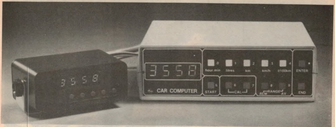
Five functions are duplicated on the remote display unit: hour.min, litres, l/100km, REM and AV (average).
