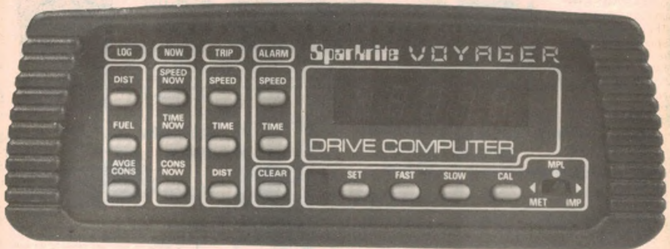
The Voyager car computer can display fuel consumption in three ways: Miles/gallon, miles/litre and litres/100km.
