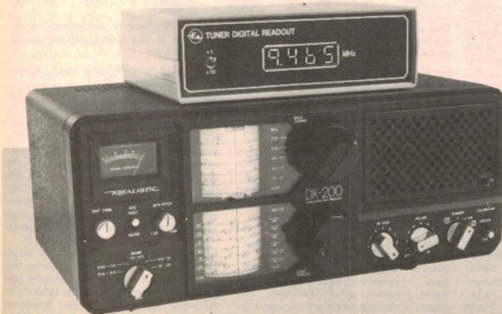
The Tuner Digital Readout can be used with broadcast-band AM tuners and communications receivers.
