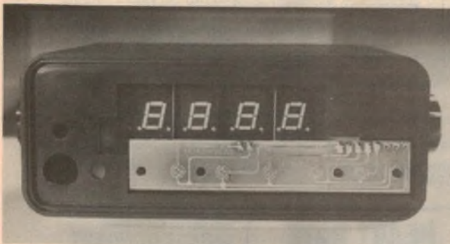
This view shows the prototype with the front panel removed to reveal the LED displays and the switch PCB.
