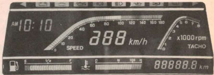
Multi-colour LCD instrument panel from Epson Corporation, Japan. Five different colours are featured: blue, green, yellow, red and black.
