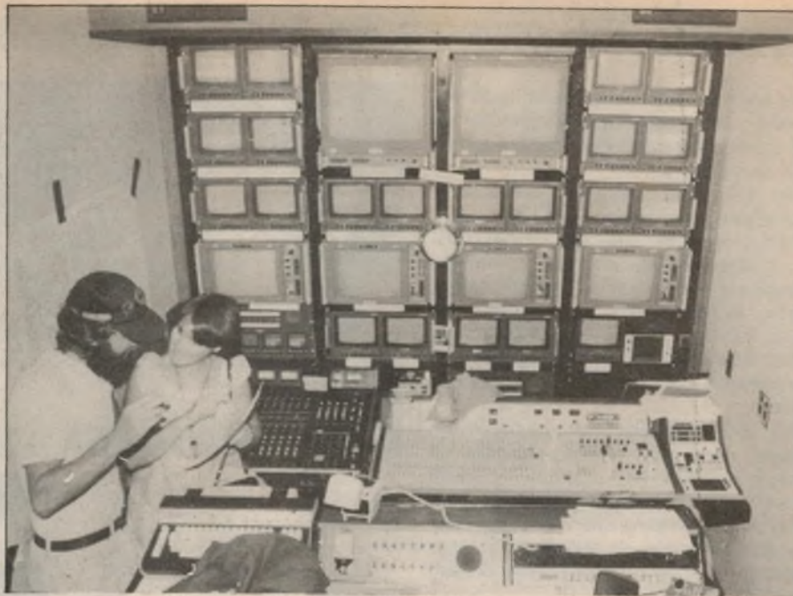
This is one of the four rooms inside the ABC's largest OB van. On the far wall are the various monitors. At the lower desk are the audio mixer (black) and the video mixer and effects unit. In the foreground, left, is the Quantafont caption console.
