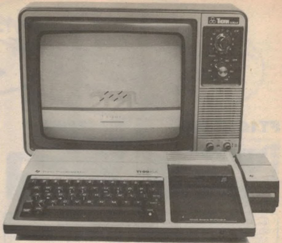
"Early Reader" program cartridge tells stories and asks the user to identify particular words and phrases. The speech synthesiser module is visible at right.
