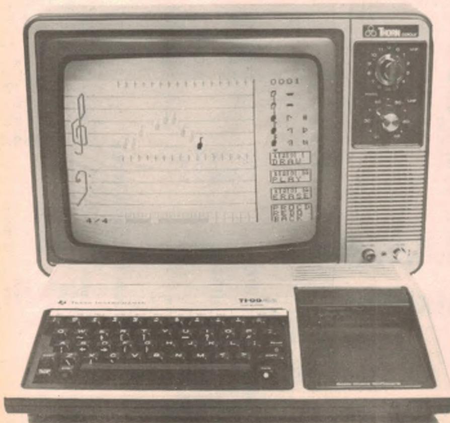
The TI-99/4A has extensive sound and graphics capabilities, as shown by the "Music Maker" cartridge. Photo was taken using a television set modified for direct video.
