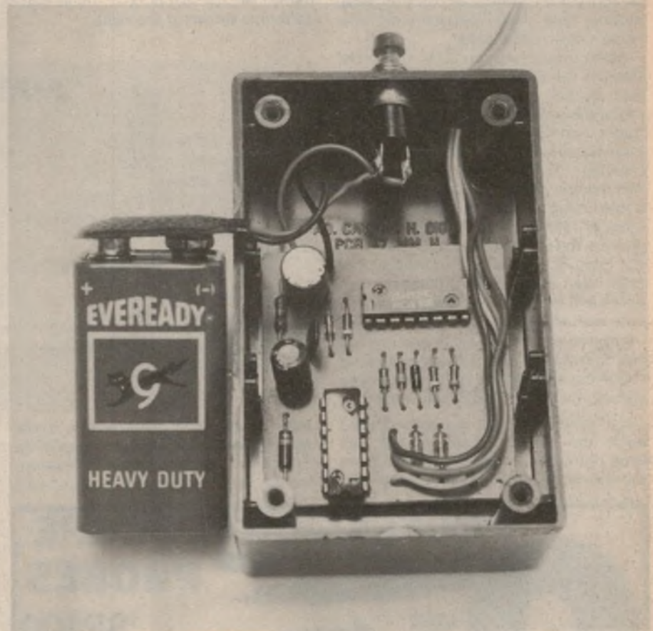
View inside the prototype, showing how the PCB fits into a small plastic utility box. The battery sits on top of the PCB and should be wrapped in plastic foam to prevent shorts.
