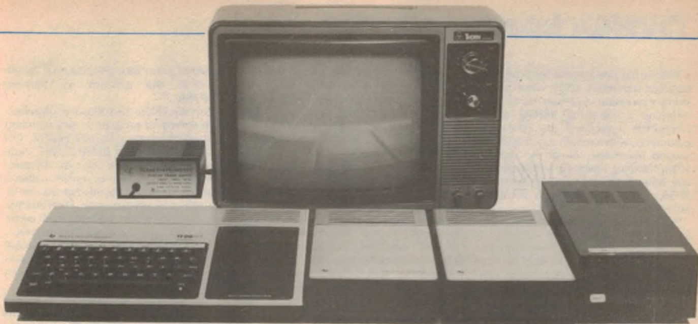
Expanded system includes 32K memory module, disk controller and disk drive. The separate power supply is on the left.
