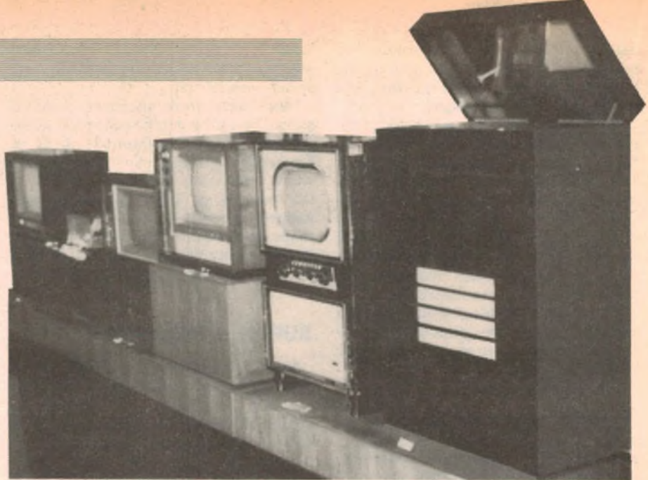
A line-up of historic television receivers at the Matsushita company museum in Osaka, Japan. In the model on the right, the picture is viewed via a 45-degree mirror beneath the lift-up lid.
