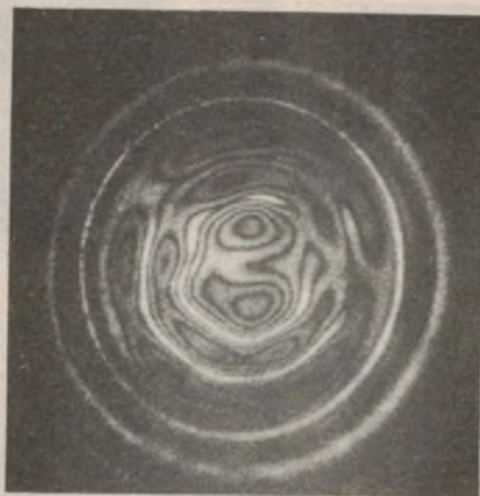
Fig. 6a: Seen through the eyes of Wharfedale's SCALP, the cone on the left has severe break-up problems while the cone on the right (Fig. 6b) is free of the effect.
