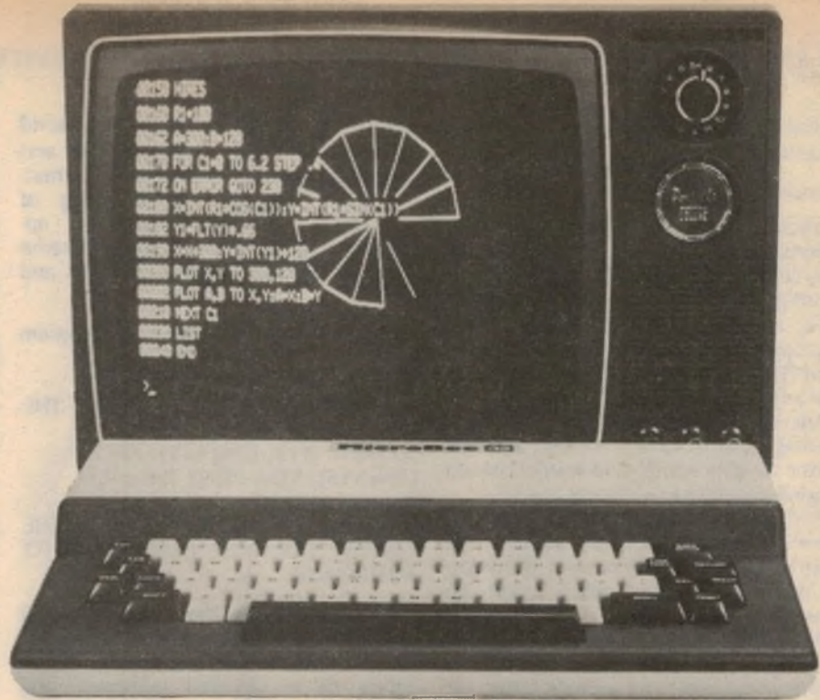
High resolution (512 x 256) graphics displays can be over-printed with text as shown here. The incomplete design results when all programmable characters have been used.
