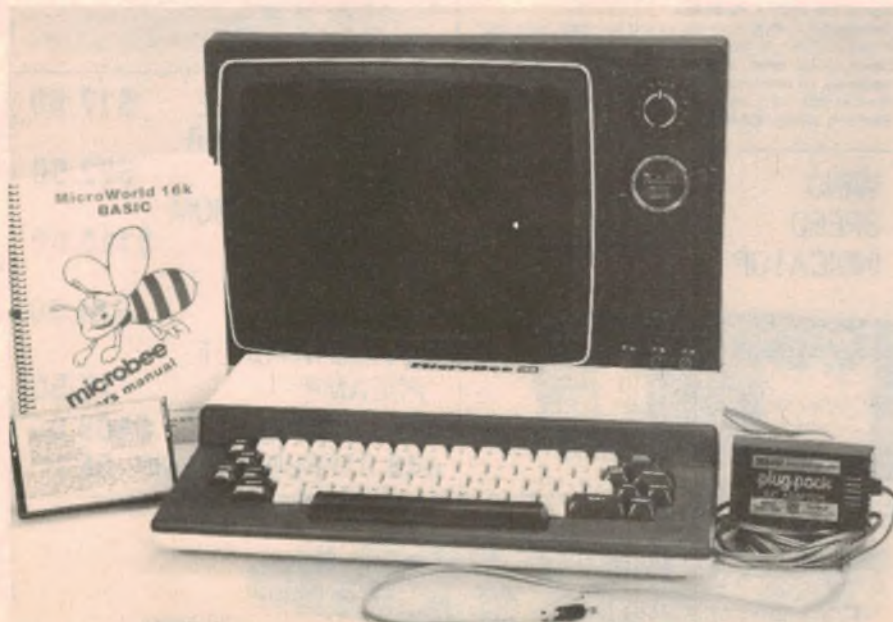
The Applied Technology MicroBee computer is supplied with a 12VAC plugpack power supply, manual and demonstration cassette. Plugs at front are for cassette recorder.
