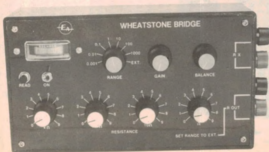
The Wheatstone Bridge can measure resistance values from 0.001\Omega to 9.999M\Omega .
