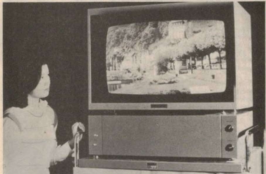
Cable may open the way for high definition television (HDTV), requiring receivers such as this NHK/Matsushita high resolution monitor.
