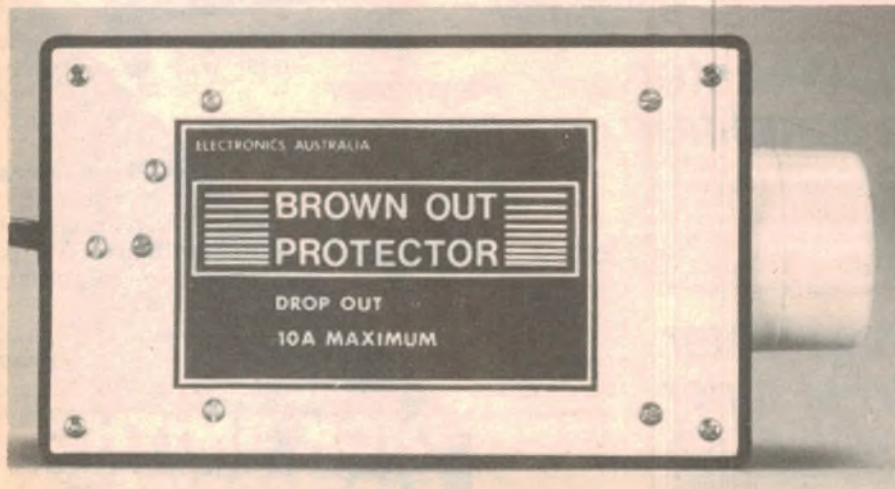
The Brown-out Protector automatically trips a relay to disconnect the load whenever the mains voltage falls below a preset level.
