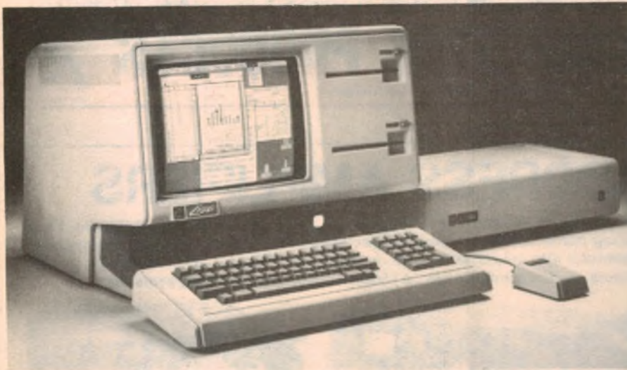
The Apple Lisa comes with built-in floppy disk drives and a 5MB hard disk. The small device at the right is the "mouse" for controlling a pointer on the screen.
