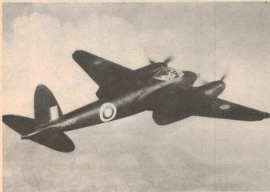
The all-black Mosquito night-fighter prototype, W4052. The radar antenna was an arrow-head design mounted in the nose between machine guns.
