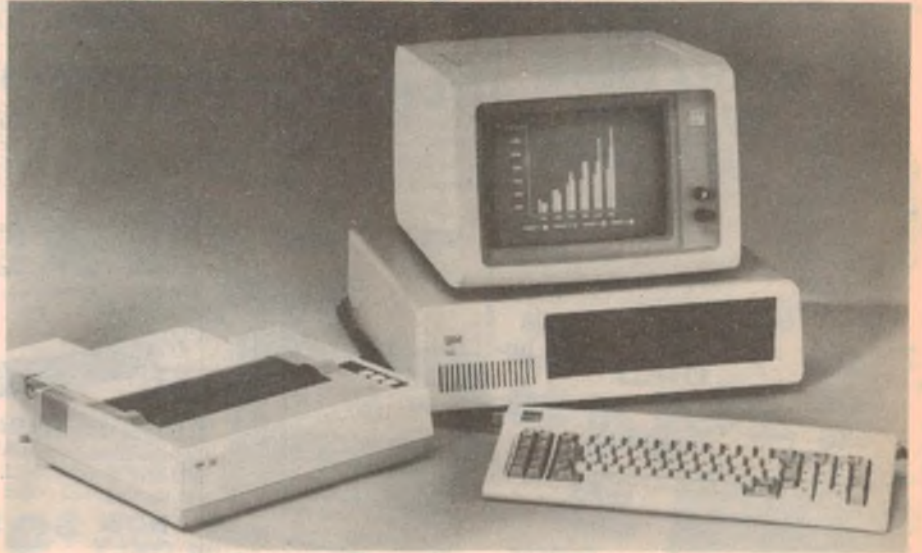
This is IBM's PC business system which includes two disc drives, B&W monitor, dot matrix printer and DOS software at a price of $6510.
