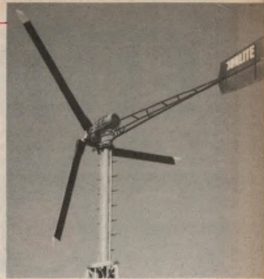
This Dunlite commercial installation provides a maximum continuous output of 2kW in a 40km/h wind and is available with a selection of output voltages. Features include a three phase alternator with solid-state regulator and an automatic feathering mechanism to protect the prop and alternator in high winds. A disc brake on the prop simplifies maintenance and installation. For further information contact Dunlite at PO Box 100, Hindmarsh, SA 5007 or offices in other states.
