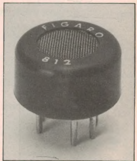
Larger-than-life size view of the Figaro TGS 812 gas sensor. The type 812 has a high sensitivity to carbon monoxide and ethanol, the latter characteristic making it suitable for use as an alcohol detector.
