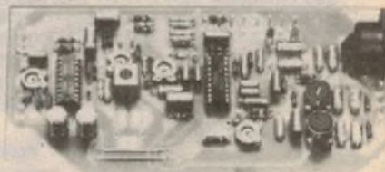
A single FM channel from just two chips.
