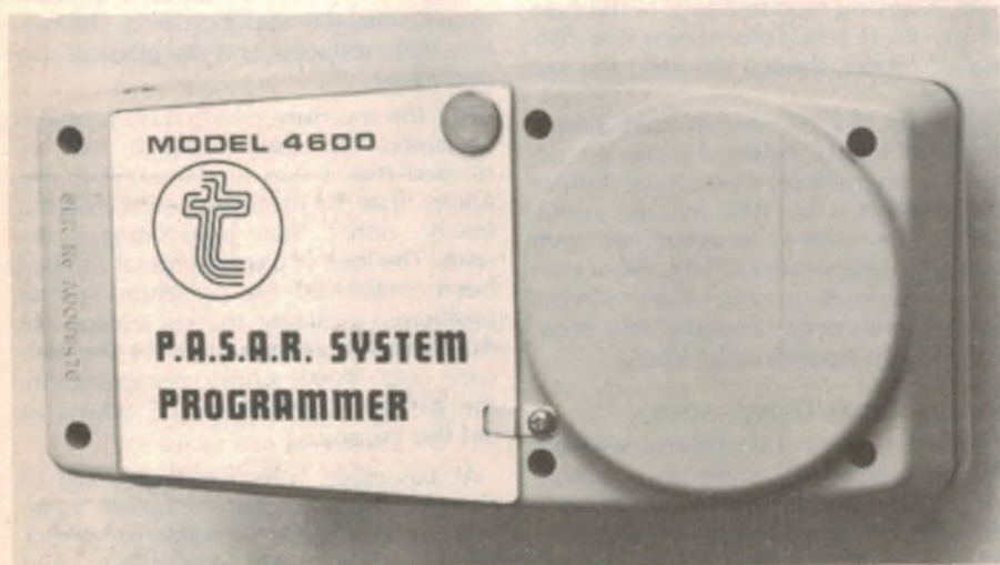
The underside of a pacemaker programmer, showing the outline of the heavy duty electromagnet which actuates a tiny reed switch in the pacemaker.
