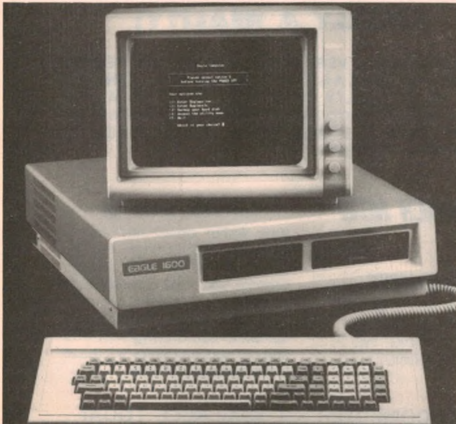
The Eagle 1600, distributed in Australia by Scomo Pty Ltd, was introduced at the DATA '83 exhibition. Features include an 8MHz 8086 processor and 10MB hard disk.
