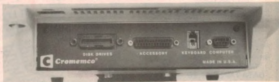
The rear of the C10 cabinet has connections for disk drives, printer, communication options, and of course, the keyboard.
