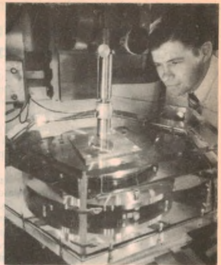
Above: a general view of the General Electric ultrasonic acoustic microscope. Shown at left is an image of a crystalline solder layer between two 30mm diameter silicon wafers.
