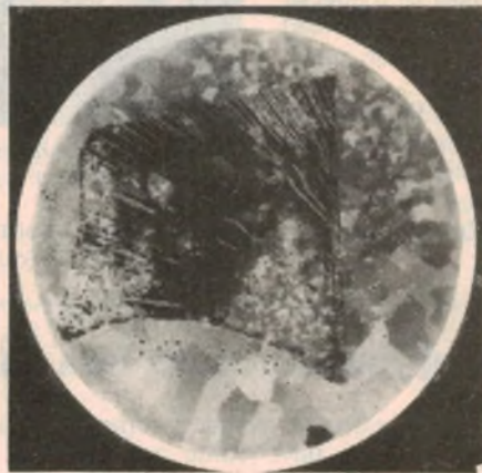
Above: a general view of the General Electric ultrasonic acoustic microscope. Shown at left is an image of a crystalline solder layer between two 30mm diameter silicon wafers.
