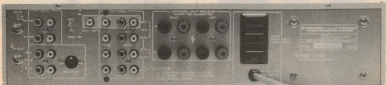
On the rear panel, the audio connections are at the left, then the video connections, with speaker terminals in the centre.
