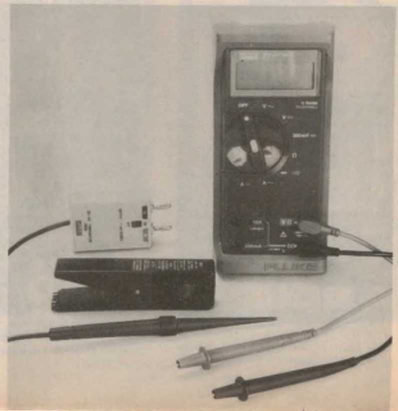
A number of accessories are available for Fluke multimeters such as these current and temperature probes.
