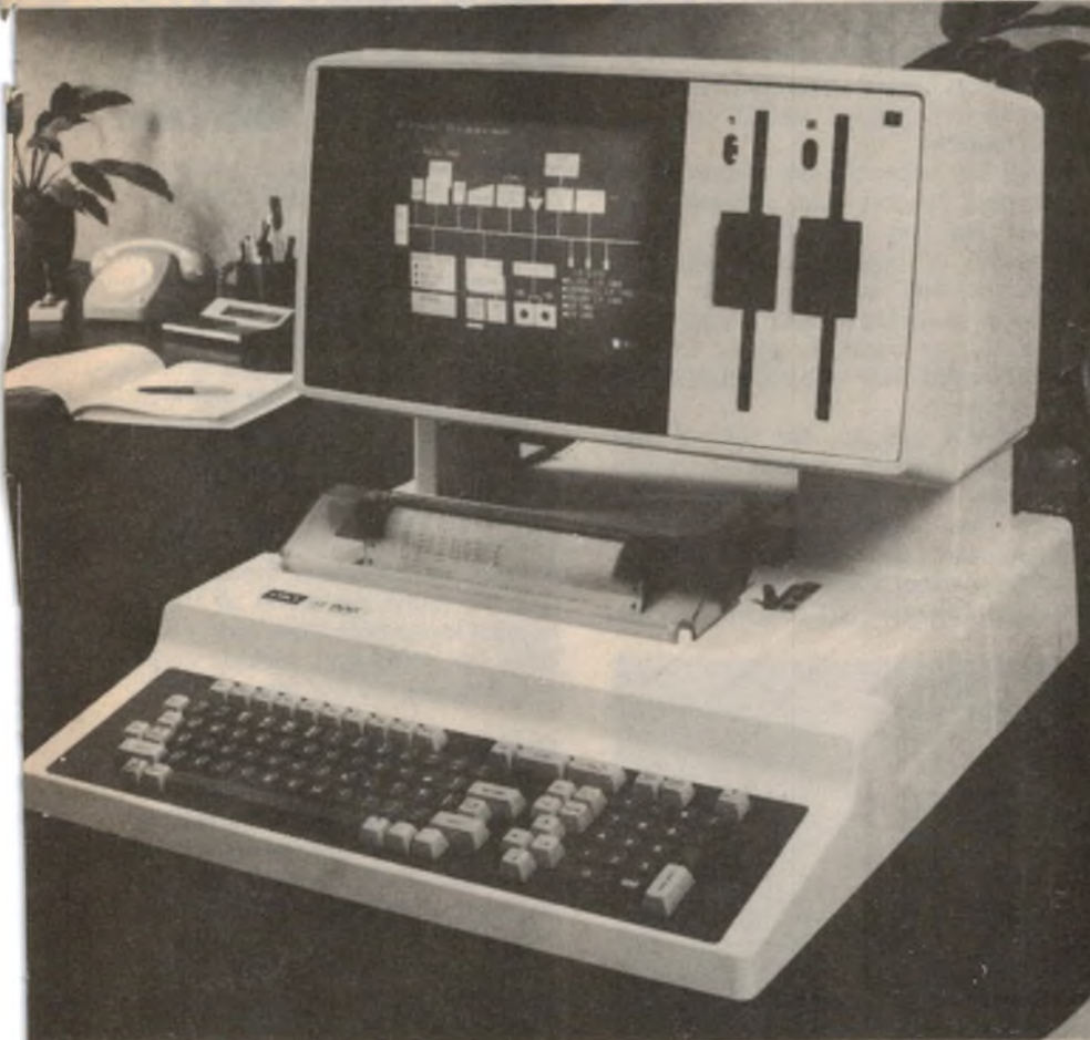
The if800 comes complete with printer, colour monitor and dual disk drives.
