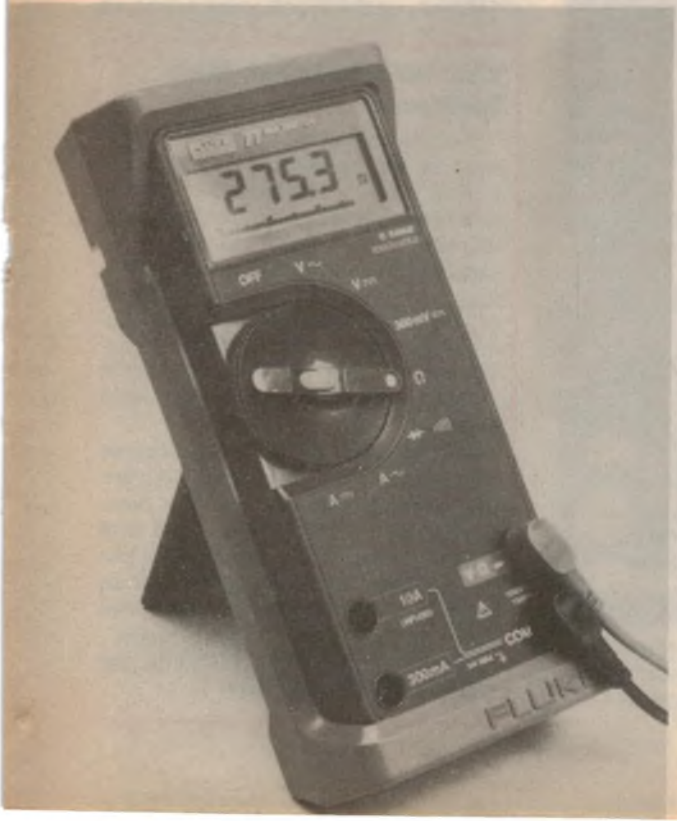
These Fluke meters are supplied with a plastic holster which can be used in a number of attitudes.
