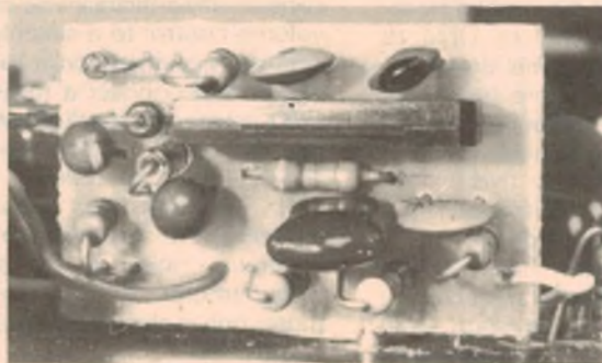
The S-meter board is mounted vertically on two PC stakes as shown at left and top left.
