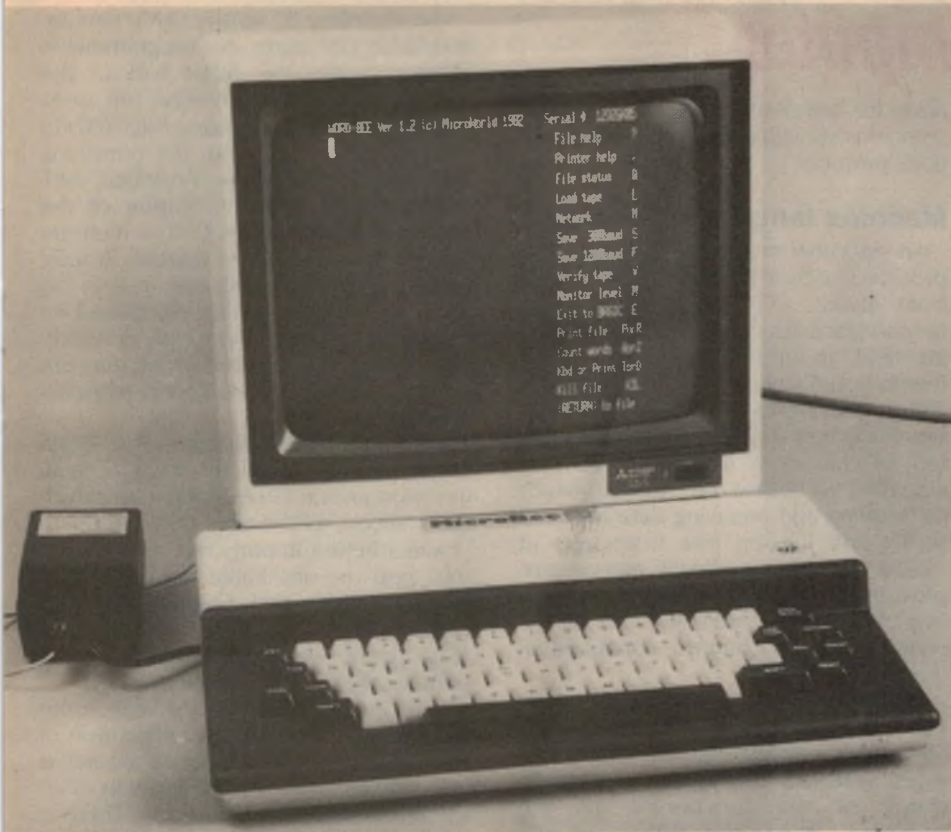
The Microbee IC in operation. On the screen is the initial WordBee menu.
