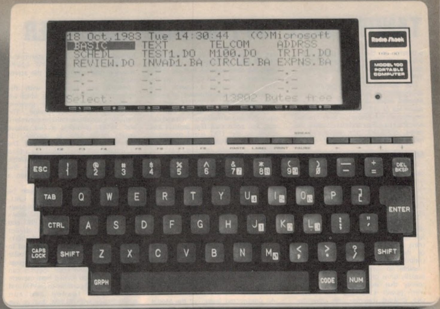
Tandy's Model 100 portable computer comes with five built-in programs and the capacity to store many more files.
