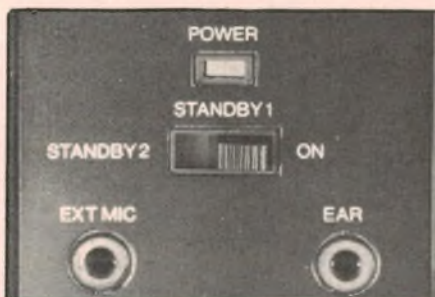
On the rear of the camera, the Standby switch and provision for external mic and monitoring earphone.
