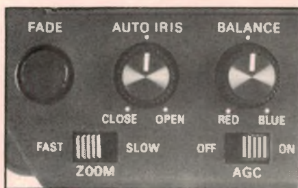
A group of picture-taking controls. The Iris knob allows compensation for very light or dark backgrounds.
