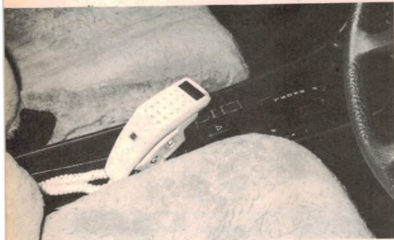
A typical handset and cradle installation in a modern car. The slightly angled mounting favours the driver's viewpoint.
