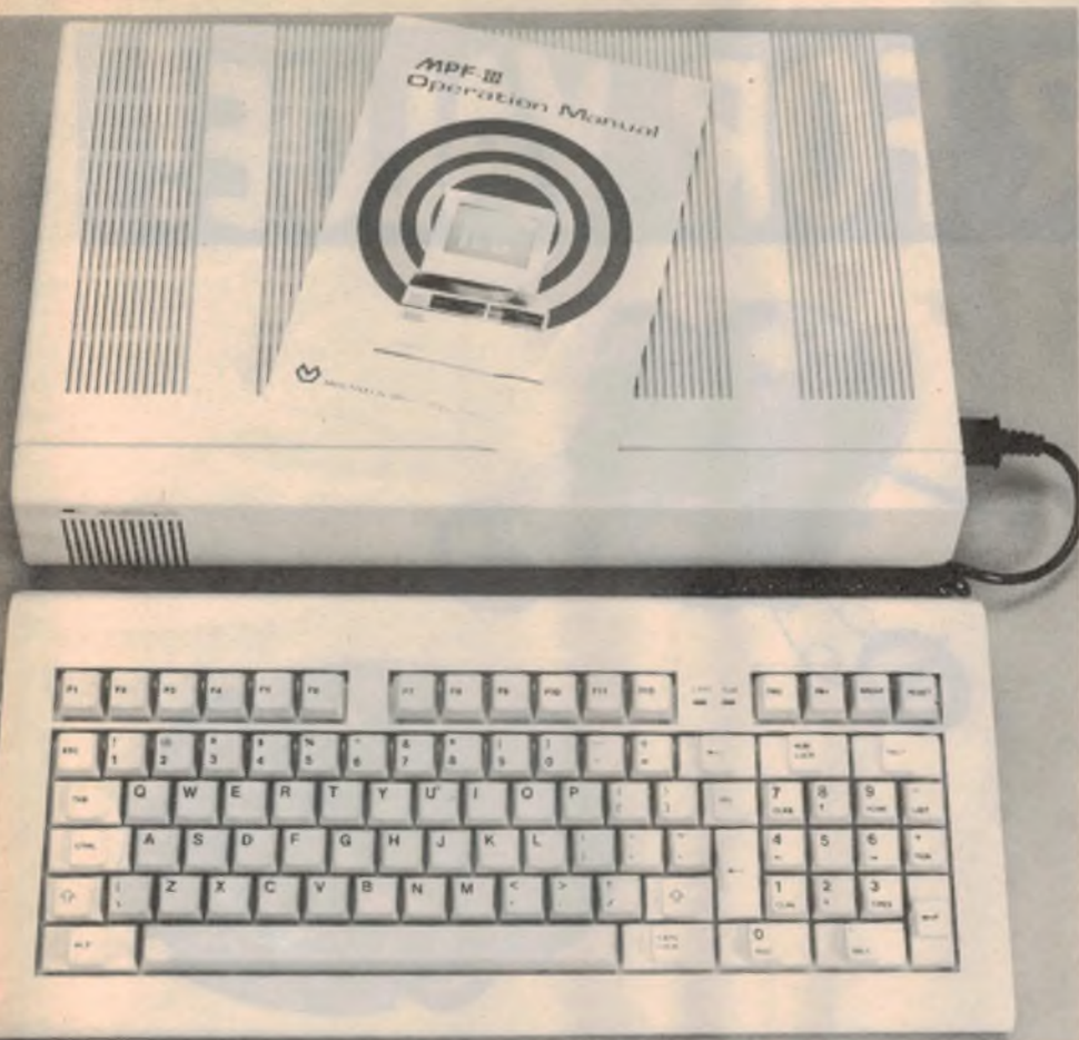
MPF-III comes in two parts: a low profile keyboard and a "system unit" which contains the dual processors, control logic and 66K of RAM.
