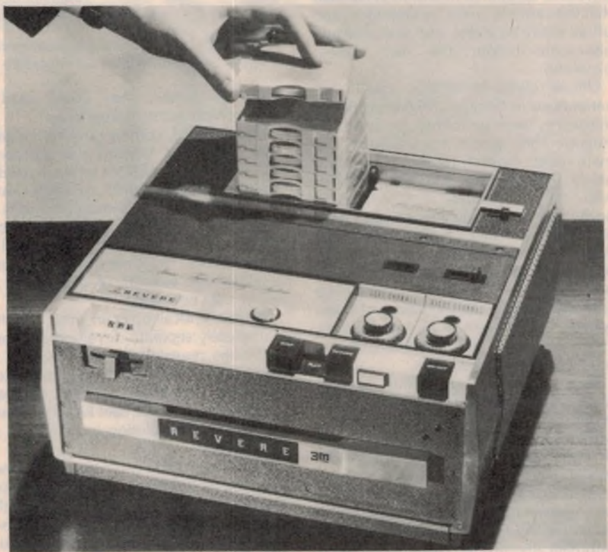
Devised jointly by CBS and 3M, this single-spool cassette system was easy to use but difficult to manufacture. It did not survive but it triggered Philips and Grundig into action.
