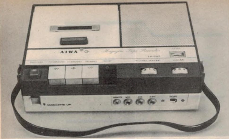
The Aiwa TP-707, claimed to be the first cassette recorder to be released in Japan. Within three months it was modified to accept the Philips cassette.
