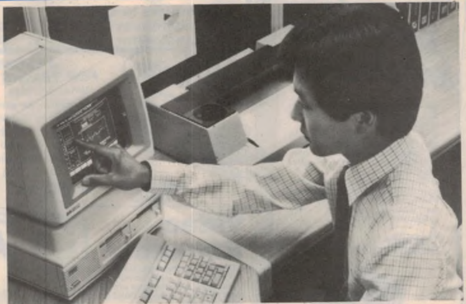
Hewlett-Packard's HP 150 runs MS-DOS and features a touch sensitive screen.
