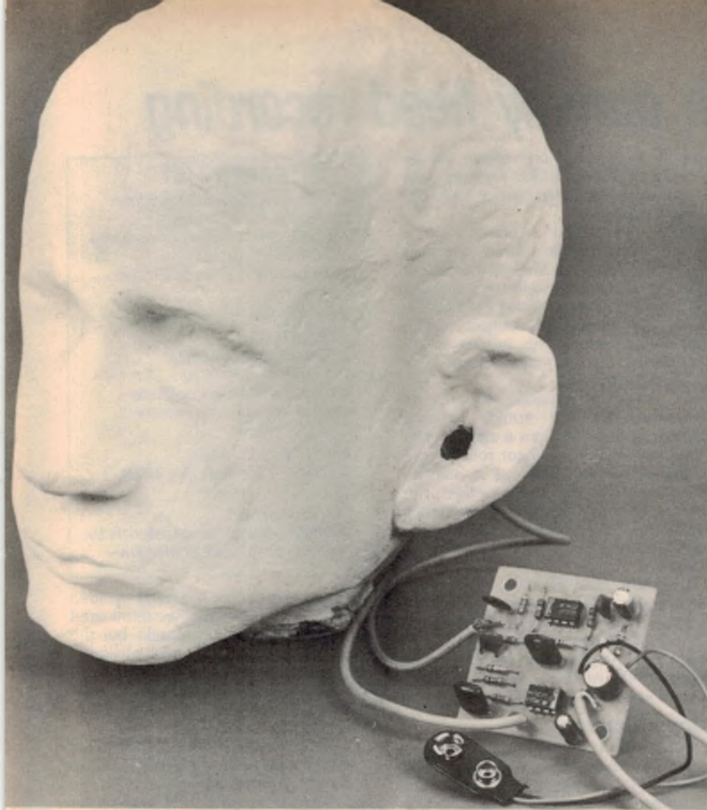
Each ear of the dummy head is fitted with an electret microphone.
