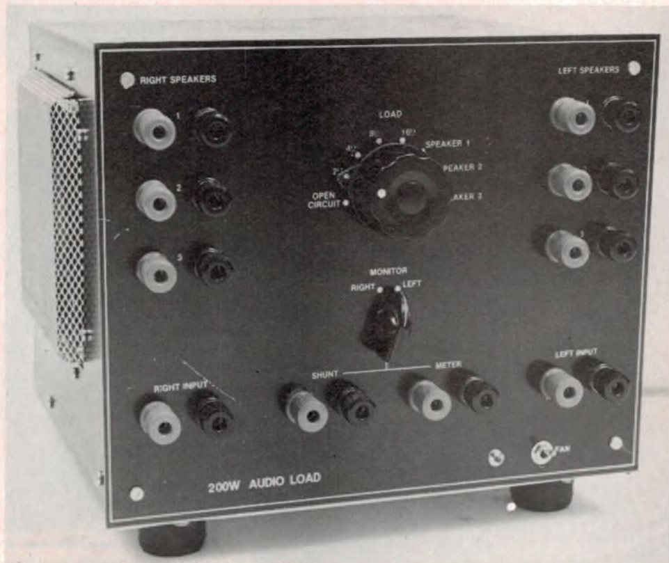
This load box provides four load resistance values. The shunt terminals enable connection of a capacitance substitution box for stability testing of amplifiers.
