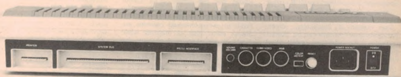
At the rear of the CAT console is an array of connectors including a printer port, expansion bus and two video outputs.
