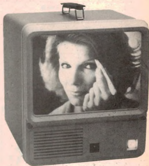
The Labelle "Showman", a traditional point-of-sale AV unit using film strip and audio tape. The screen size is about the same as that of the VS-1.
