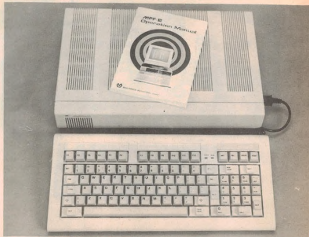
The MPF-III provides Apple II compatibility in a compact, low profile design with detachable keyboard. Features include an 80-column display, 64K RAM, printer and cassette ports and an Apple compatible hardware expansion slot. As yet however, no colour graphics are available. The February 1984 issue of Electronics Australia has a review of the system.
