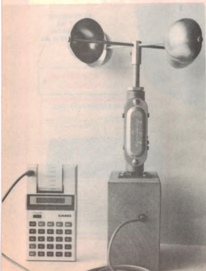
The complete data logger, comprising commercial anemometer and modified Casio printing calculator.
