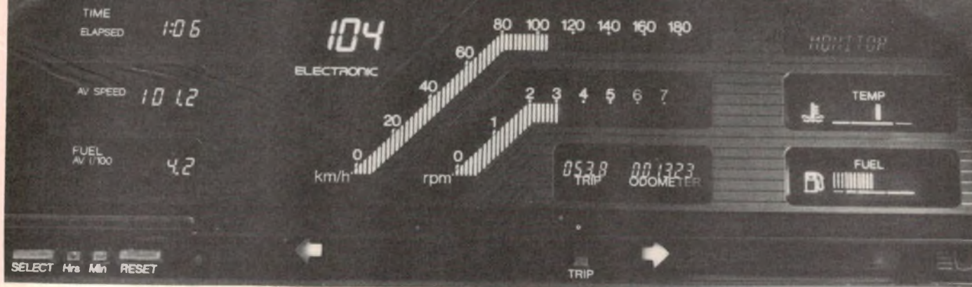
A photographer's through-the-wheel view of the Calais all-electronic instrument panel. A number of indicators along the bottom edge are il-
