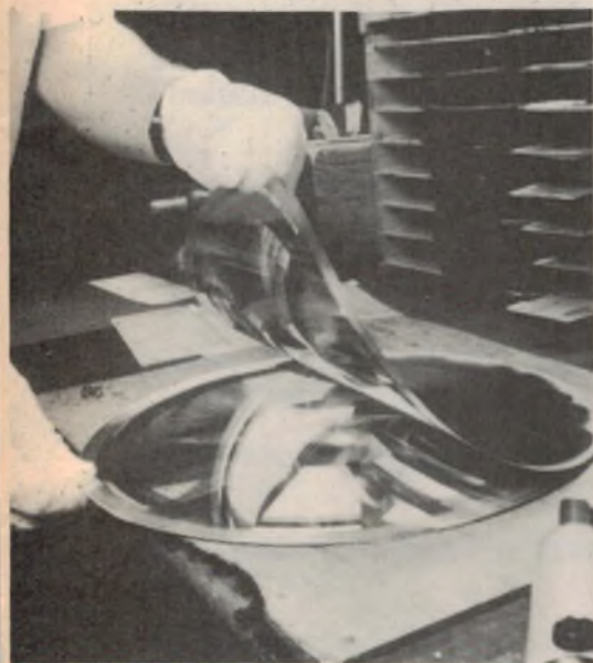
Below: Thanks to the use of a parting agent, the metal stamper can be stripped from the copper master after electroplating.
