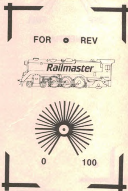
This artwork for the walkaround throttle fits a standard UB5 zippy box (28 x 54 x 83mm).
