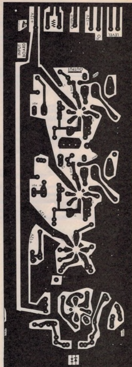
Fig. 6: full size PC pattern for current to voltage converter of Fig. 5 (see page 70).
