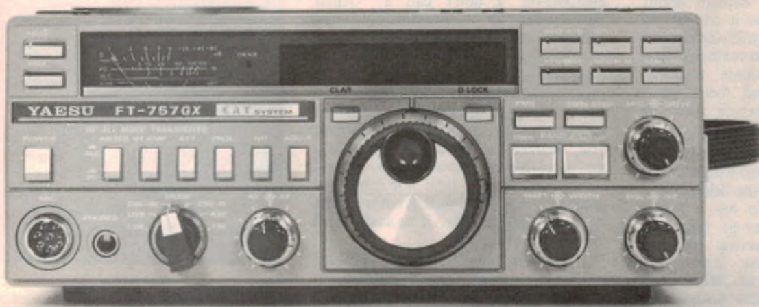
A typical piece of amateur commercial equipment. The Yaesu FT-757GX is a MF/HF transceiver covering all amateur bands from 1.8 to 30MHz. The transmitter is rated at 100W in SSB, CW, and FM, and the receiver gives continuous coverage. (Photo from Dick Smith Electronics.)
