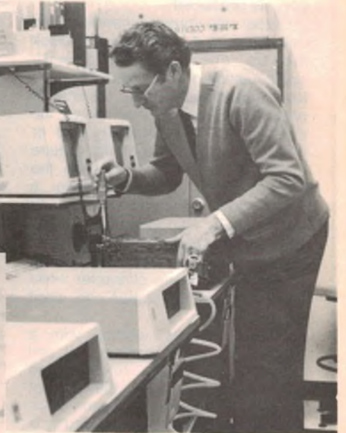
At left, a PC undergoes diagnostic checks while above, more PCs with option cards are tested at varying voltages.
