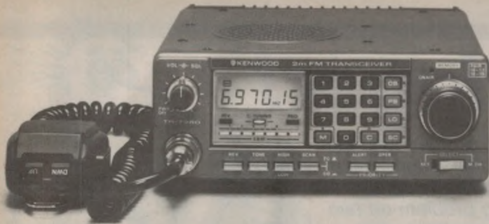
For the VHF enthusiast this Kenwood TR-7950 two metre transceiver is suitable for either station or mobile use. It covers from 144 to 148MHz in 5kHz steps, operates in the FM mode, and is rated at 50W. (Photo from Trio-Kenwood (Aust) Pty Ltd.)
