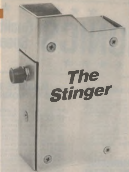
The "Stinger". Note the folded panel for the sides and the separate front panel.
