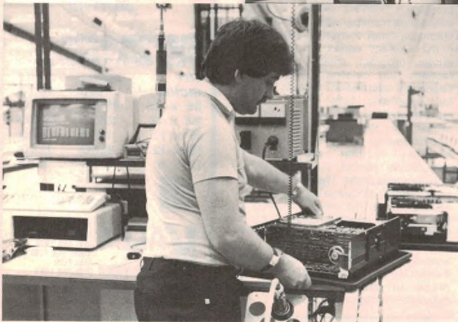
At left, a PC undergoes diagnostic checks while above, more PCs with option cards are tested at varying voltages.
